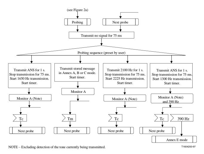
Figure 2b/V.18 - Automode probing
