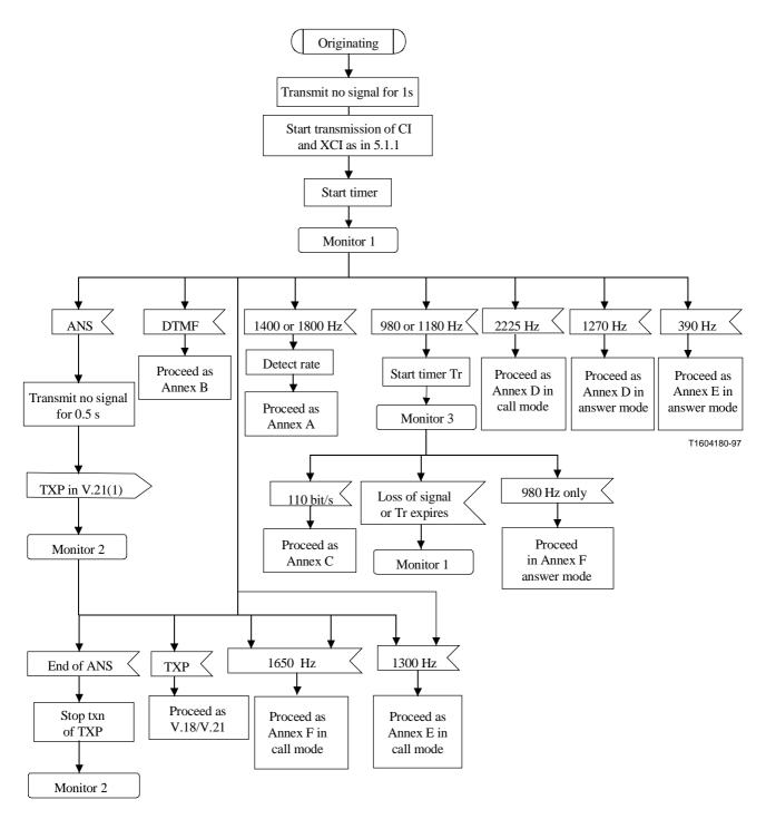
Figure 1/V.18 – Start-up procedure in the originating V.18 DCE with automoding to existing types of text telephone without use of V.8 bis
