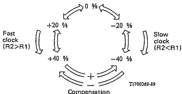
*Note 1* – Phase measurements are given relative to R1 by the formula: Phase = phase(R2) – phase(R1).
