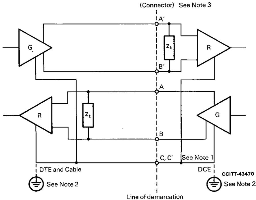
Note 1 – The zero volt reference interchange point C, C' may be interconnected via the signal ground conductor.
