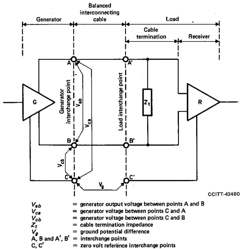
Note 1 – Two interchange points are shown. The output characteristics of the generator, excluding any interconnecting cable, are defined at the “generator interchange point”. The electrical characteristics to which the receiver must respond are defined at the “load interchange point”.
