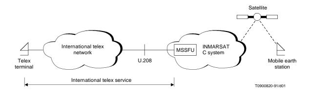
Figure 1/U.208 – General model for interworking between the international telex service and the INMARSAT C system
