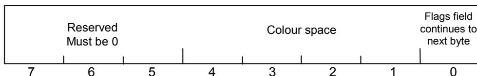
Figure AMD3-4 – Structure of the first byte of colour palette flags
