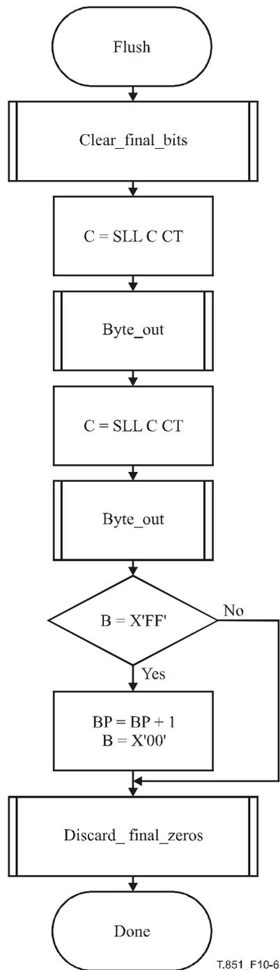
**Figure 10-6/T.851 – Flush procedure for Q15-coder**
