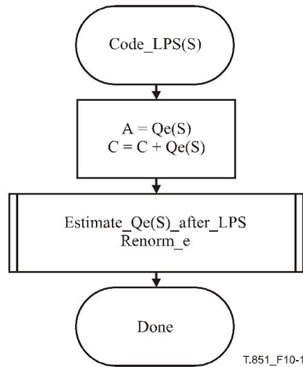
**Figure 10-1/T.851 – Code\_LPS(S) procedure for Q15-coder**
