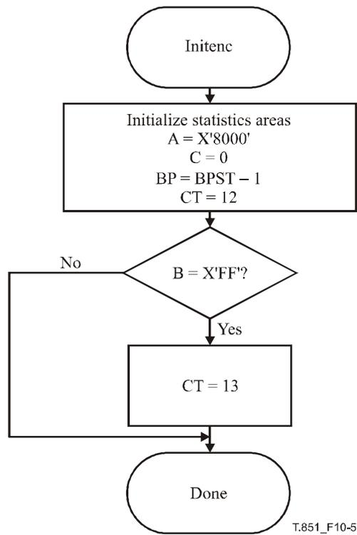
**Figure 10-5/T.851 – Initialization of the encoder for Q15-coder**
