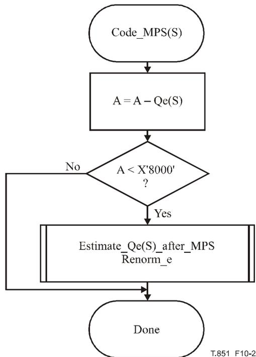
**Figure 10-2/T.851 – Code\_MPS(S) procedure for Q15-coder**
