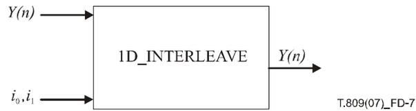
Figure D.7 – Parameters of the 1D\_INTERLEAVE procedure
