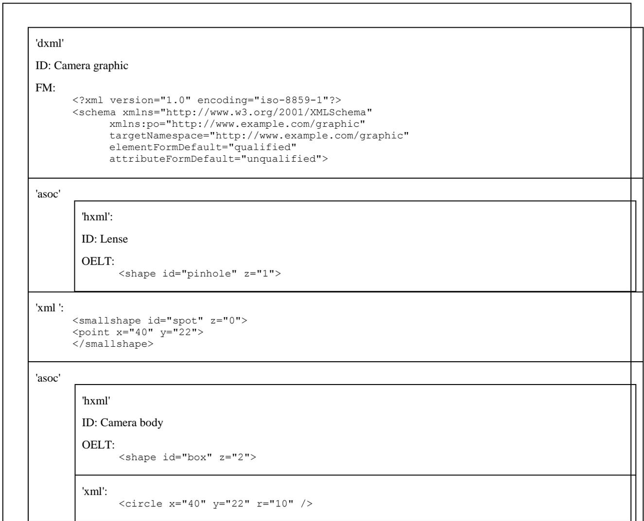
Figure M.49 – Example Box layout for a Decomposed XML box
