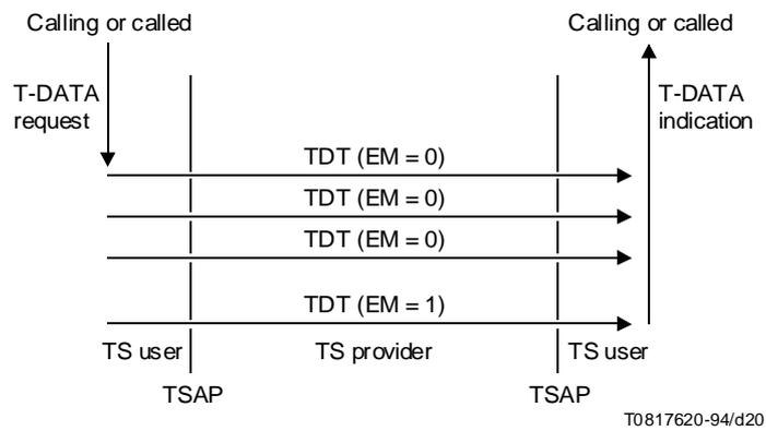
NOTE – This is one method of realizing segmenting/reassembling.
