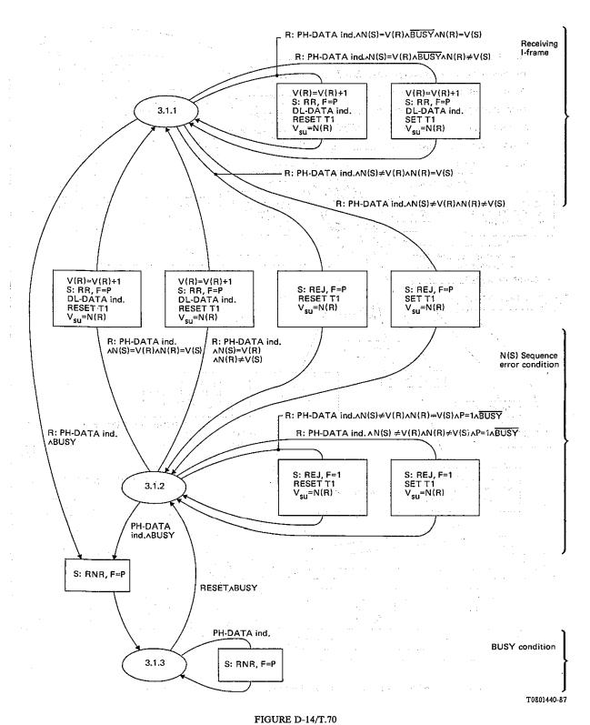
State transition diagram HDLC (3.1 information transfer phase, I-frame acknowledgement)
