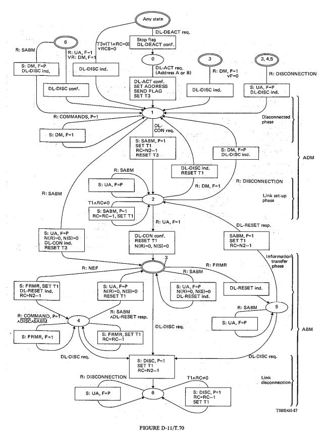
State transition diagram HDLC (Data link control)
