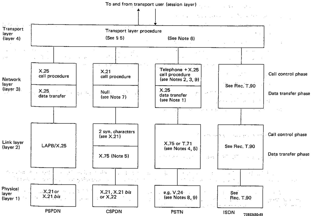
*Note 1* – The X.25 network layer procedure is introduced to ease interworking with PSPDNs.
