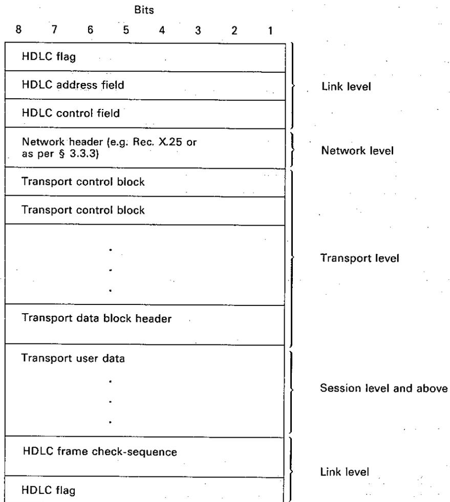
*Note* — This figure does not imply that a transport data or control block will fit within a single network data block.
