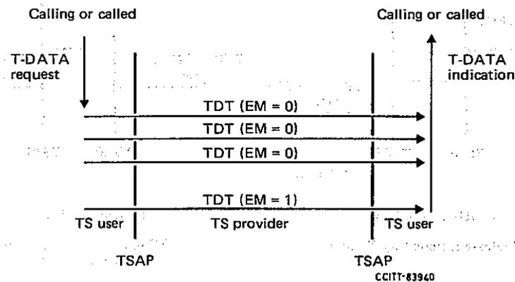
*Note* – This is one method of realizing segmenting/reassembling.
