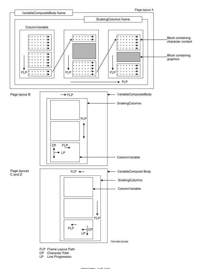
FIGURE 8/T.505 Examples of the layout of snaking columns
