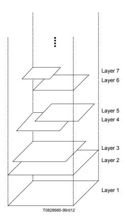
Figure A.1/T.44 – Mask and image layers in N-layer stripe
