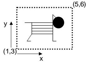
The picture above is imaged into the basic layout object as shown. The heavy border represents the boundary of the basic layout object.
