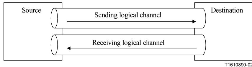
**Figure B.1/T.38 – A pair of unidirectional channels**
