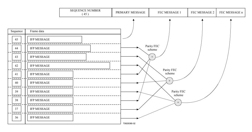
Figure C.3/T.38 – Generating multiple FEC messages to protect against burst errors
