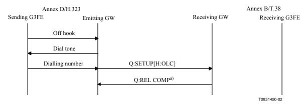
Annex B/T.38 implementation rejects connection by sending Q.931: RELEASE COMPLETE when it receives SETUP message without fastStart element.
