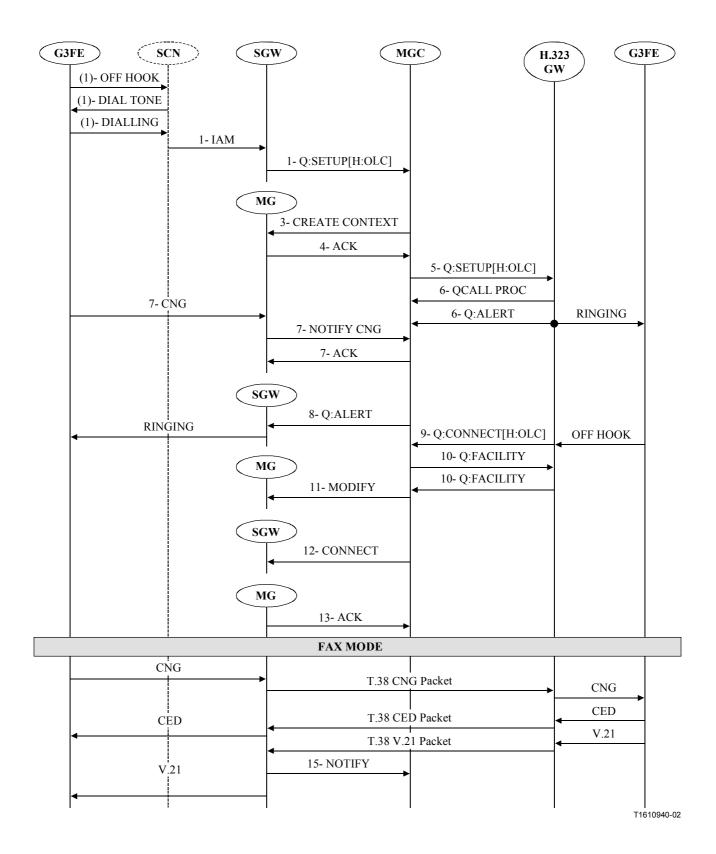
Figure III.2/T.38 – Fax only call setup between H.248 and an H.323 endpoint
