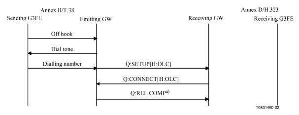
Annex B/T.38 implementation rejects connection by sending Q.931: RELEASE COMPLETE when it receives CONNECT message without fastStart element in response to its SETUP message with fastStart element.
