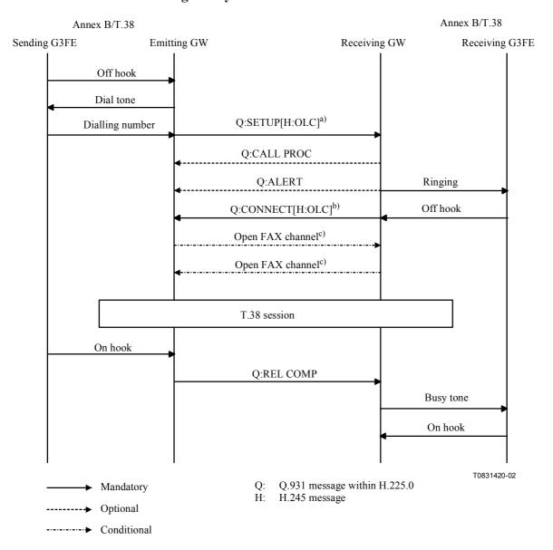
a) SETUP contains Setup-UUIE, which includes fastStart element that is linked to OpenLogicalChannel (OLC) of ITU-T Rec. H.245.
