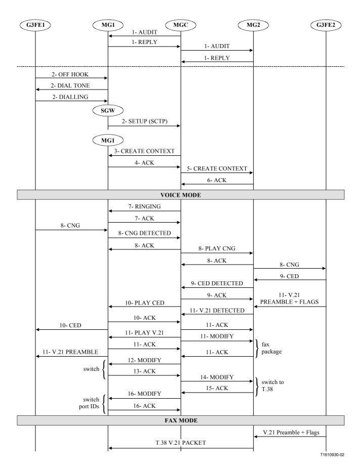
Figure III.1/T.38 – Voice to fax call setup with H.248 endpoints
