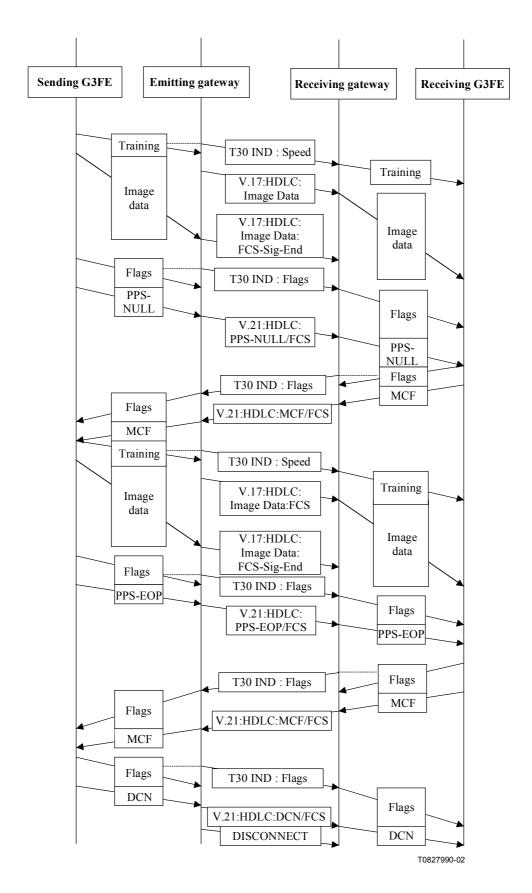
Figure I.1/T.38 – Two Group 3 facsimile devices communicating through gateways (sheet 2 of 2)
