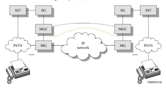
Figure E.1/T.38 – Typical decomposed model
