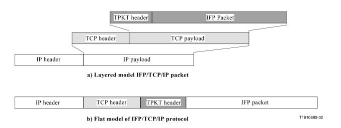
Figure 4/T.38 – High-level TCP/TPKT/IP packet structure
