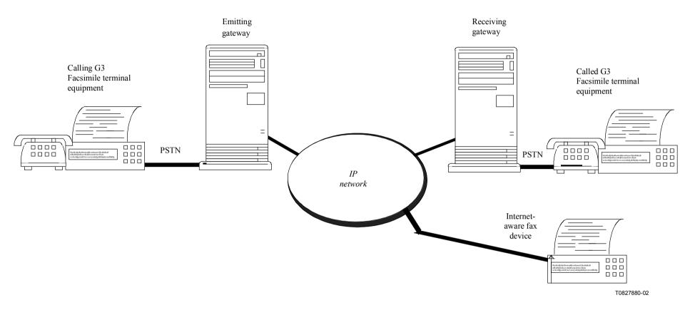
Figure 1/T.38 – Model for facsimile transmission over IP Networks
