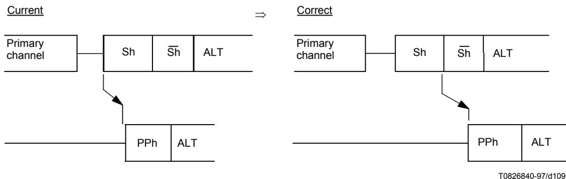
**F.4.6 The portion of Figure 27/V.34 shown should be changed to conform with the text**
