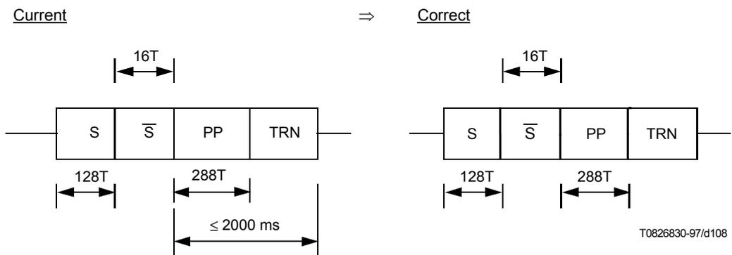
**F.4.5 The portion of Figure 26/V.34 shown should be changed to conform with the text**
