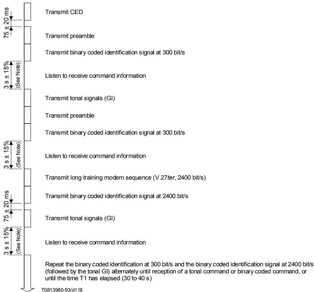
NOTE – For manual receivers using the binary coded procedure, this delay should be  $4.5 \text{ s} \pm 15\%$ .
