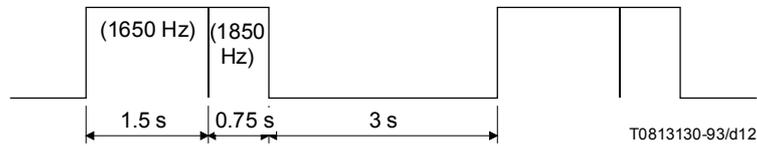
NOTE – Tolerances: timing  $\pm 15\%$ ; frequency  $\pm 6$  Hz.
