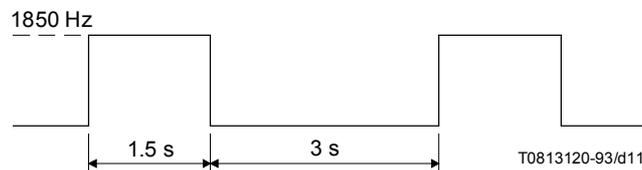
NOTE – Tolerances: timing  $\pm 15\%$ ; frequency  $\pm 6$  Hz.
