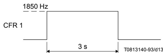
NOTE – Tolerances: timing  $\pm 15\%$ ; frequency  $\pm 6$  Hz.
