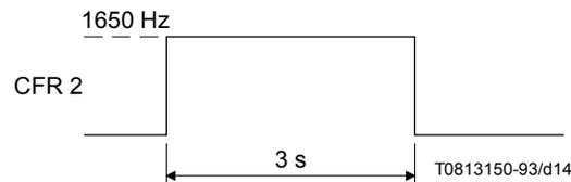
NOTE – Tolerances: timing  $\pm 15\%$ ; frequency  $\pm 6$  Hz.
