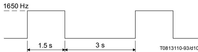
NOTE – Tolerances: timing  $\pm 15\%$ ; frequency  $\pm 6$  Hz.
