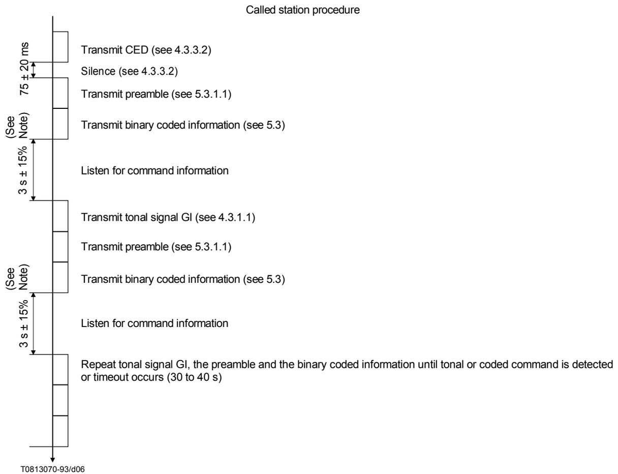
NOTE – For manual receivers using the binary coded procedure, this delay should be 4.5 s ± 15%.
