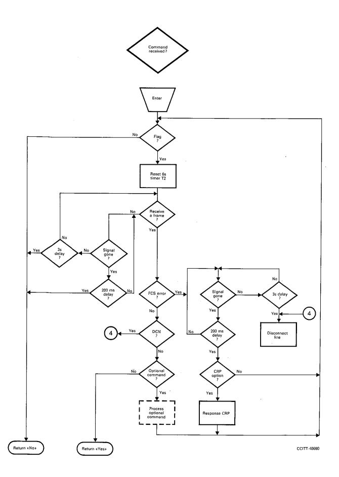
Interworking between the standard mode (300 bit/s) and the recognized optional mode (2400 bit/s) for the binary coded handshaking procedure is provided by an alternating method.
