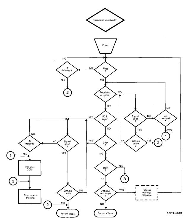
T4 = 4.5s  $\pm$  15%, for manual units T4 = 3.0s  $\pm$  15%, for automatic units
