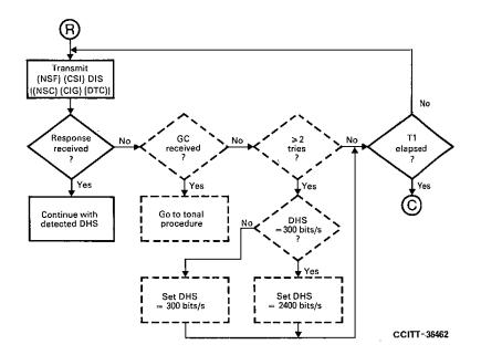
Note – The station listens to a response at 300 bits/s (2400 bit/s) after transmitting a command at 300 bit/s (2400 bit/s) and continues with the detected DHS.
