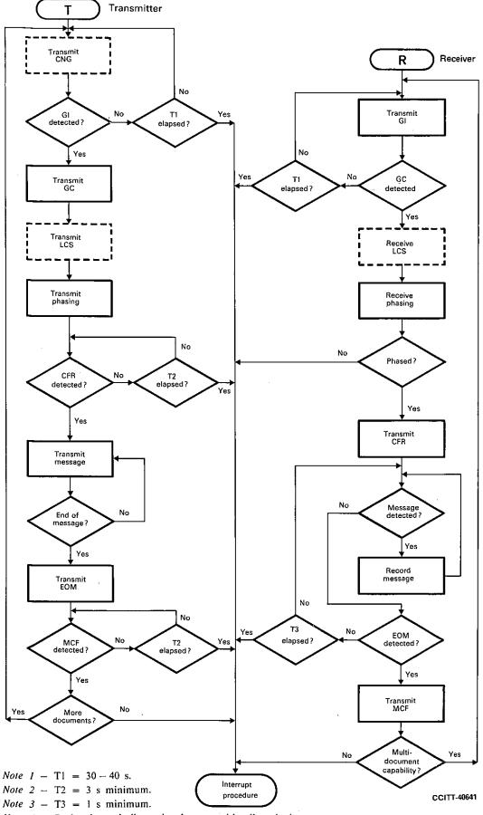
Note 4 - Broken boxes indicate signals not used in all methods.
