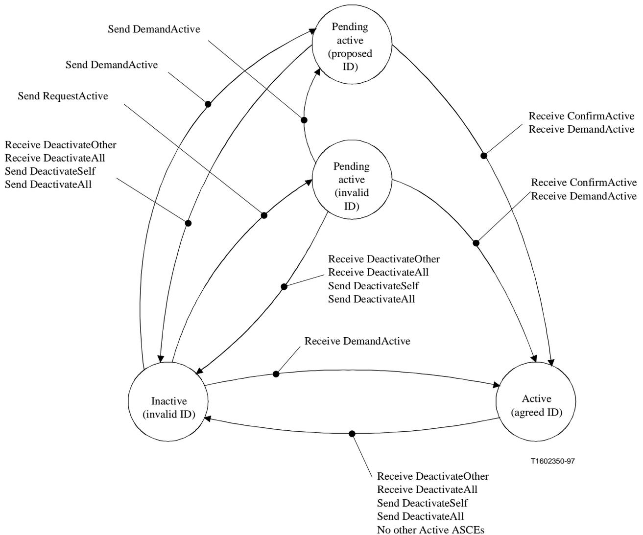
**Figure 5/T.128 – ASCE state transitions and share identifier management (Legacy mode)**
