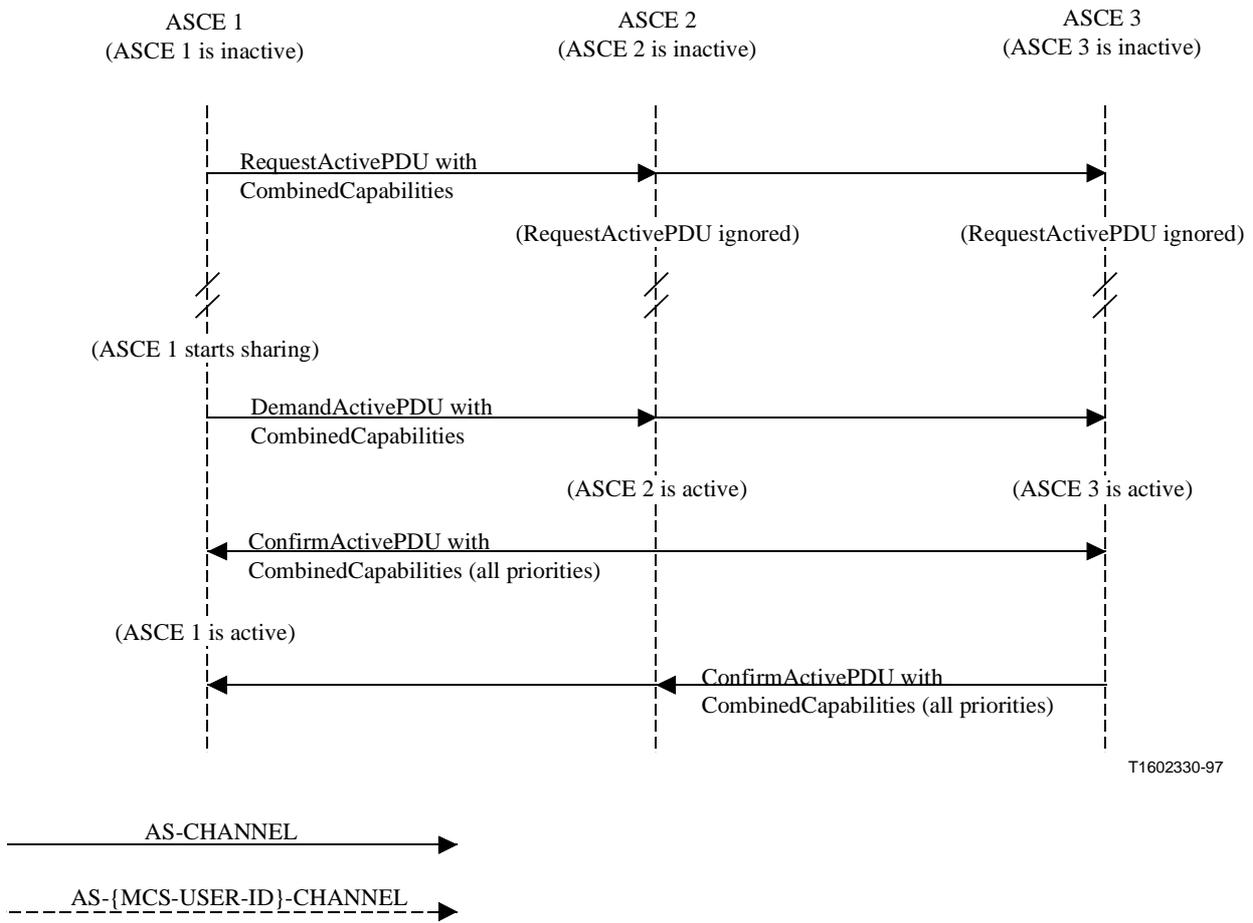
**Figure 3/T.128 – Successfully activating three ASCEs (Legacy mode)**
