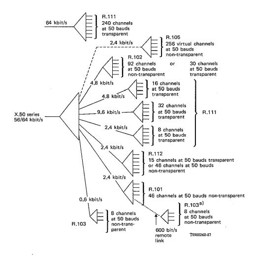
a) The R.103 remote multiplexer may be connected to an R.101, R.112 or an R.102 multiplexer. In this example, the eight remote link channels are included in the 46 channels of the R.101 multiplexer.
