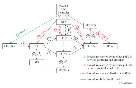
Figure 8-1 – Signalling procedure of parallel SFC
