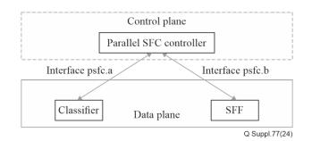
Figure 7-1 – The interface reference model of parallel SFC
