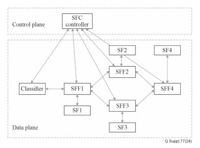
Figure 6-2 – An example of partial parallel SFC
