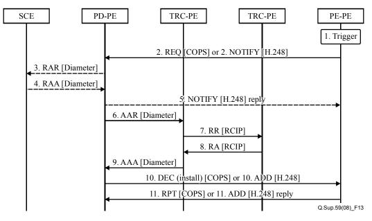
1) PE-PE receives a trigger for sending a COPS REQ or an ITU-T H.248 NOTIFY (see Note) message. This trigger could be an UE-initiated explicit QoS request for resource reservation and commitment towards the PE-PE through dedicated path-coupled transport QoS signalling.
