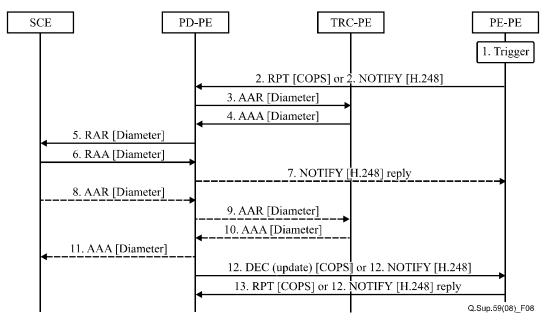
1) PE-PE receives a trigger for sending a COPS RPT or an ITU-T H.248 NOTIFY (see Note) message towards PD-PE. This trigger could be a failure that affects an existing service (e.g., interface failure).
