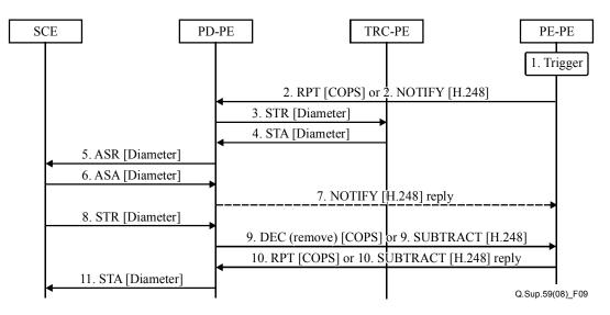
1) PE-PE receives a trigger for sending a COPS RPT or an ITU-T H.248 NOTIFY (see Note) message towards PD-PE. This trigger could be a failure that affects an existing service (e.g., interface failure).
