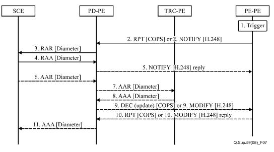
PE-PE receives a trigger for sending a COPS RPT or an ITU-T H.248 NOTIFY (see Note) message towards PD-PE. This trigger could be a certain traffic condition which needs to be reported in accordance with a service previously requested by the PD-PE.
