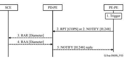
PE-PE receives a trigger for sending a COPS RPT or ITU-T H.248 NOTIFY (see Note) message. This trigger could be an UE-initiated explicit QoS request for resource commitment to the PE-PE through dedicated path-coupled transport QoS signalling.
