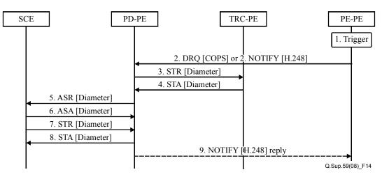
1) PE-PE receives a trigger for sending a COPS DRQ or an ITU-T H.248 NOTIFY (see Note) message towards PD-PE. This trigger could be an UE-initiated explicit QoS request for resource release towards the PE-PE through a dedicated path-coupled transport QoS signalling.
