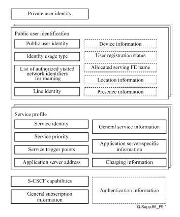
Figure 9-1 – Example of service user data in the IP multimedia subsystem
