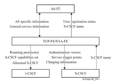
Figure II.1 – Example of data flow of service user data in the IMS
