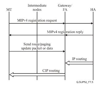
Figure 7-5 – Call flow for CIP with MIPv4
