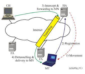
Figure 7-1 – Basic operation of MIPv4
