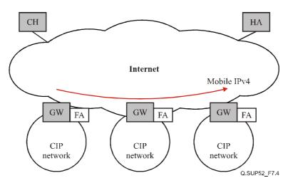
Figure 7-4 – CIP with MIPv4 for MM
