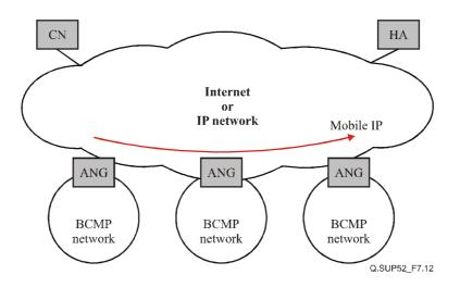
Figure 7-12 – Architecture of BCMP with MIP for MM
