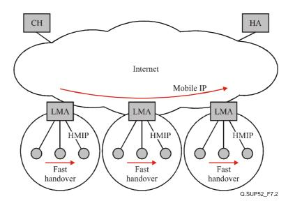
Figure 7-2 – MIP and its extensions for MM
