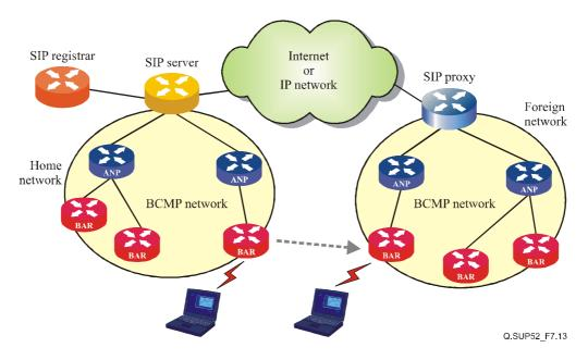
Figure 7-13 – Architecture of BCMP with SIP for MM
