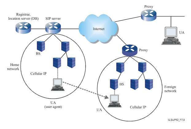
Figure 7-6 – Architecture of CIP with SIP
