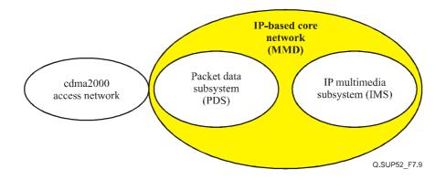
Figure 7-9 – Simplified architecture of ANSI-41 evolved all-IP MMD core network with cdma2000 access network
