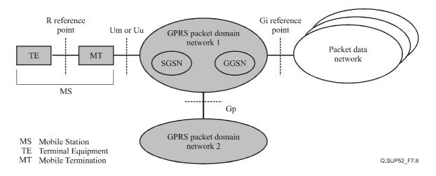
Figure 7-8 – Architecture for packet data service (GPRS system)
