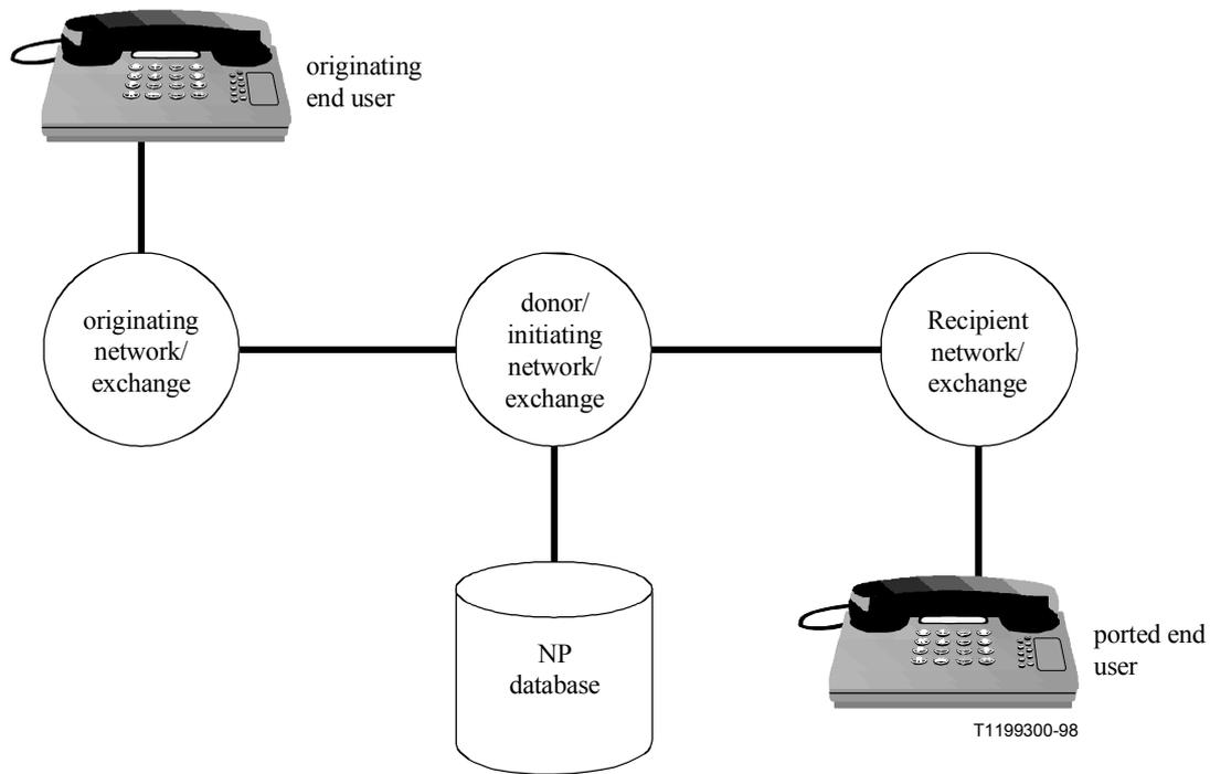
**Figure 3 – PNCC-SPP configuration – Identical donor and initiating networks/exchanges**
