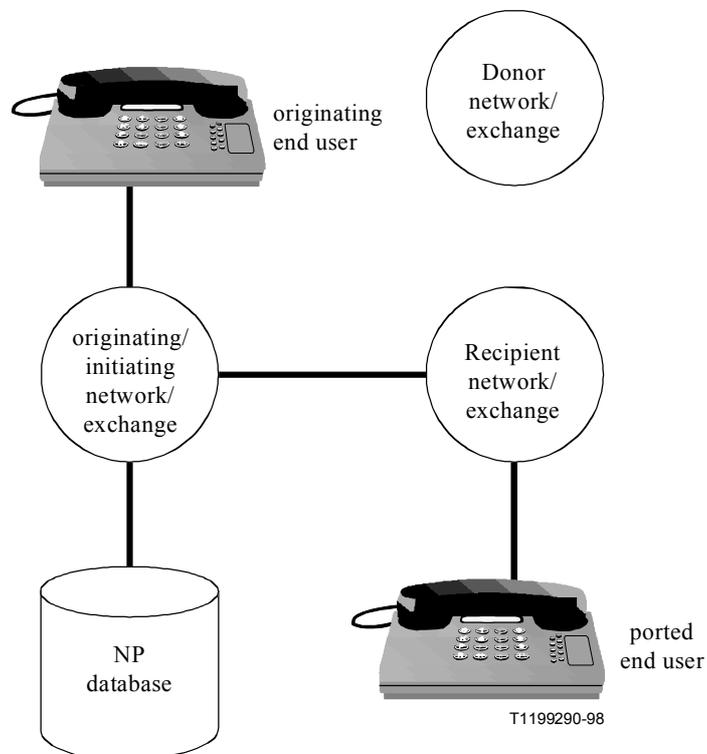
**Figure 2 – PNCC-SPP configuration – Identical originating and initiating networks/exchanges**
