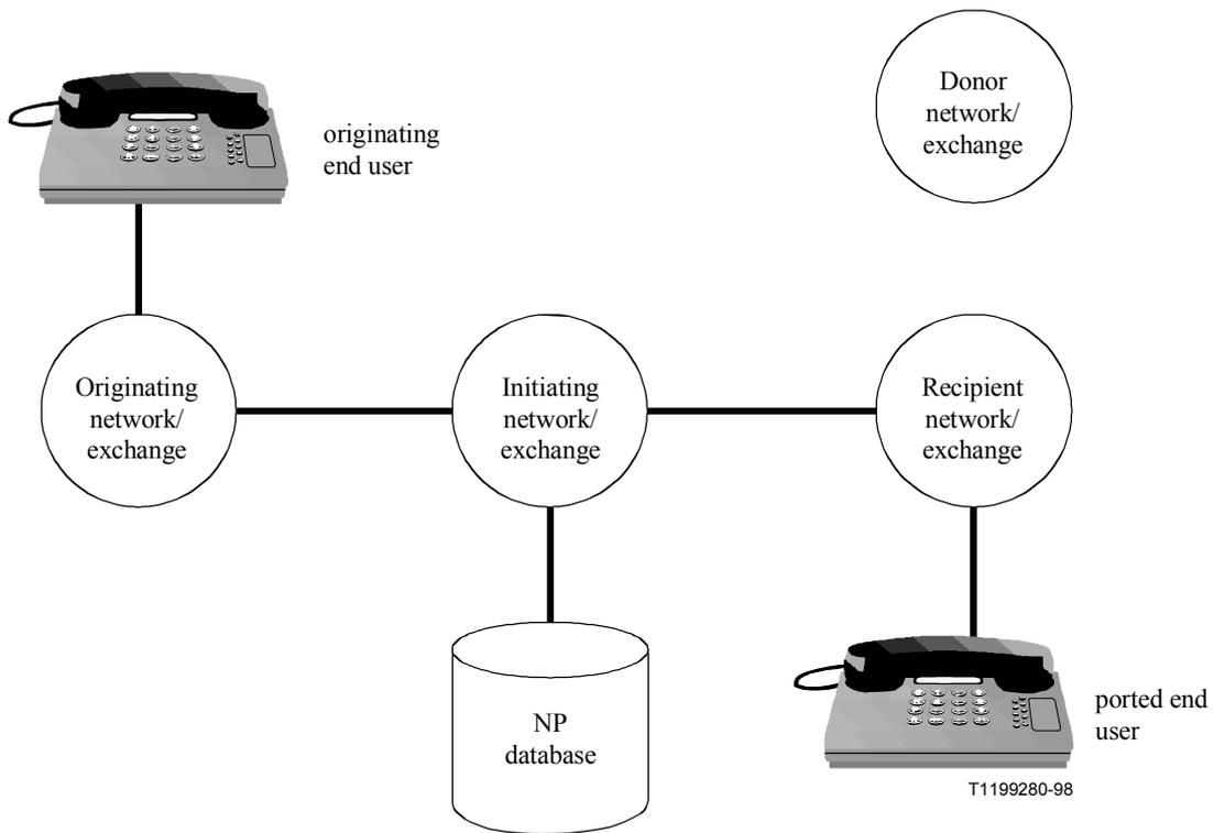
**Figure 1 – PNCC-SPP configuration – Separate originating, initiating, donor networks/exchanges**
