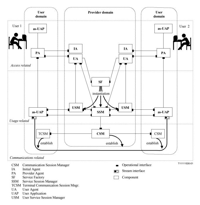
Figure 8-3 – Example of User-Provider roles using service components
