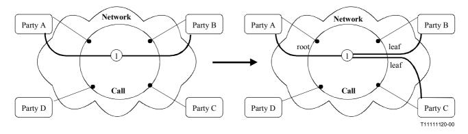
Figure 8-1 - Call and Bearer Transition for addition of a new party to an existing connection
