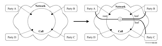
Figure 7-7 – Call and Bearer Transition for addition of a new type 2 connection to an existing call
