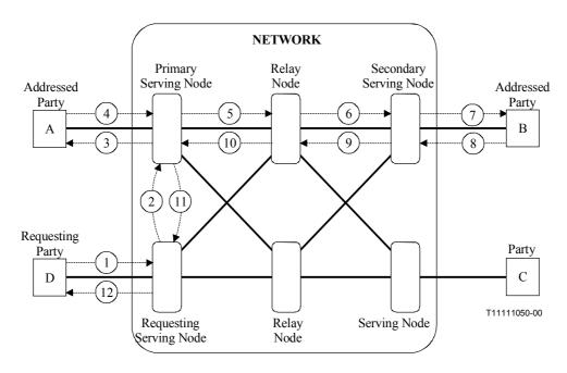
Figure 7-2 – Point-to-point Network Connection – Type 1 between A and B Third Party – No Negotiation – No Look Ahead – No Notification
