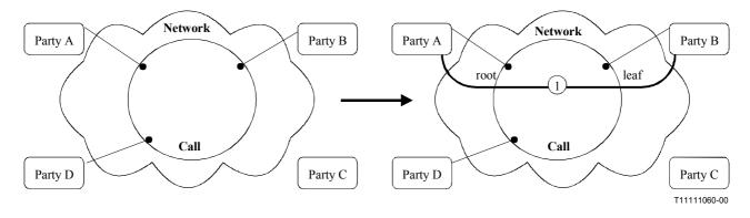
Figure 7-3 – Call and Bearer Transition for addition of a new type 1 connection to an existing call
