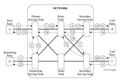
Figure 7-8 – Point-to-multipoint Network Connection (Type 2 between A, B and C) – Third Party – With Negotiation – No Look ahead – No Notification
