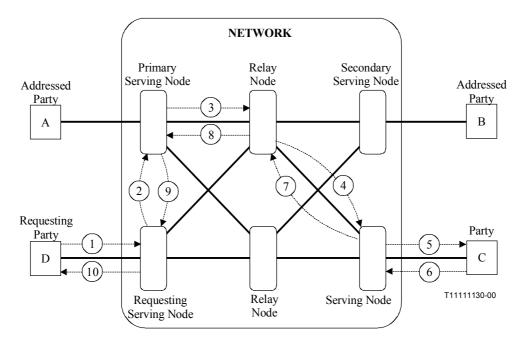
Figure 8-2 – Point-to-point Network Connection exists between A and B – Third Party D requests addition of existing Party (C) – No Negotiation – No Look Ahead – No Notification
