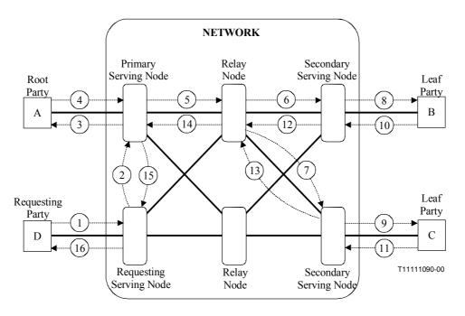
Figure 7-6 – Point-to-multipoint Network Connection (Type 2 between A, B and C) – Third Party – No Negotiation – No Look ahead – No Notification
