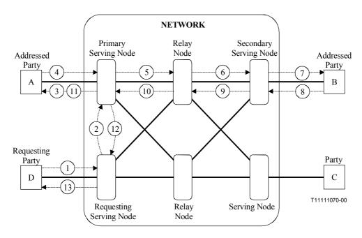
Figure 7-4 – Point-to-point Network Connection (Type 1 between A and B) – Third Party – With Negotiation – No Look ahead – No Notification
