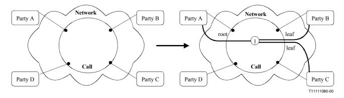
Figure 7-5 – Call and Bearer Transition for addition of a new type 2 connection to an existing call
