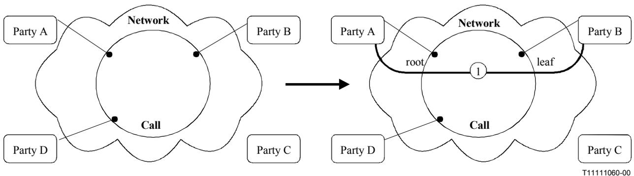
**Figure 7-3 – Call and Bearer Transition for addition of a new type 1 connection to an existing call**
