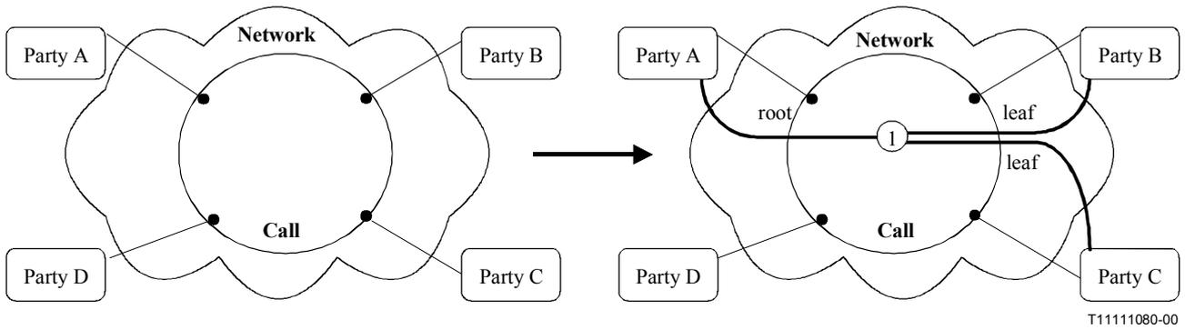
**Figure 7-5 – Call and Bearer Transition for addition of a new type 2 connection to an existing call**
