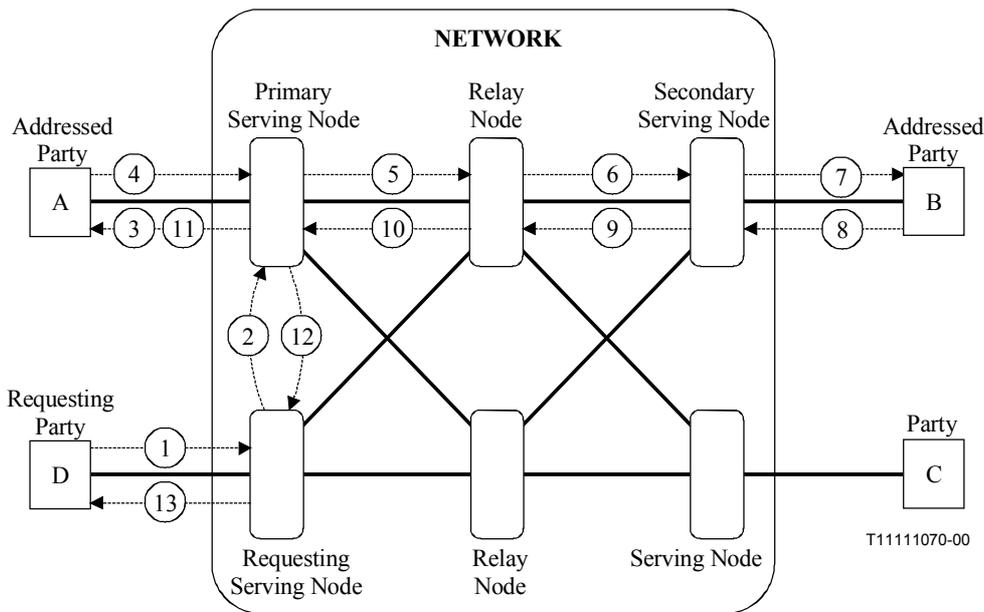
**Figure 7-4 – Point-to-point Network Connection (Type 1 between A and B) – Third Party – With Negotiation – No Look ahead – No Notification**
