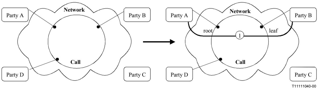
**Figure 7-1 – Call and Bearer Transition for addition of a new type 1 connection to an existing call**
