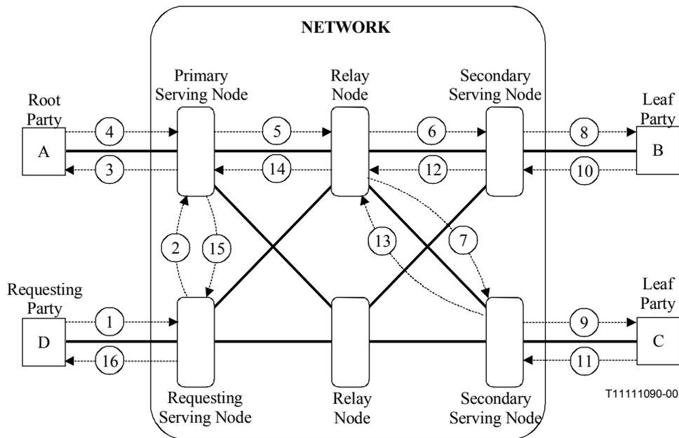
**Figure 7-6 – Point-to-multipoint Network Connection (Type 2 between A, B and C) – Third Party – No Negotiation – No Look ahead – No Notification**
