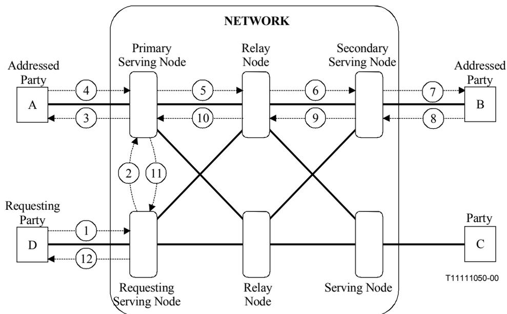
**Figure 7-2 – Point-to-point Network Connection – Type 1 between A and B
