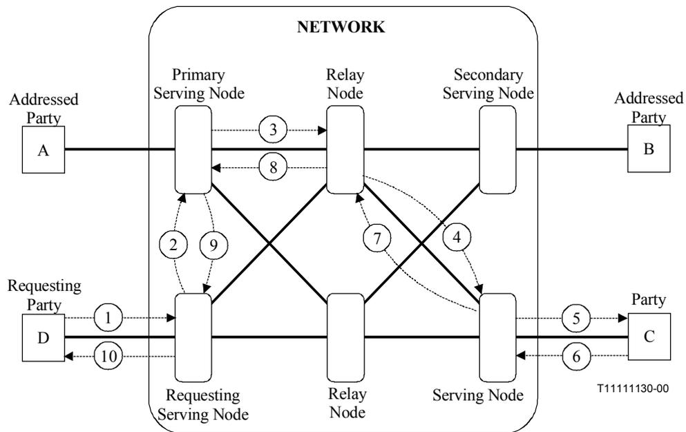
**Figure 8-2 – Point-to-point Network Connection exists between A and B – Third Party D requests addition of existing Party (C) – No Negotiation – No Look Ahead – No Notification**
