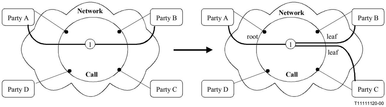
**Figure 8-1 – Call and Bearer Transition for addition of a new party to an existing connection**
