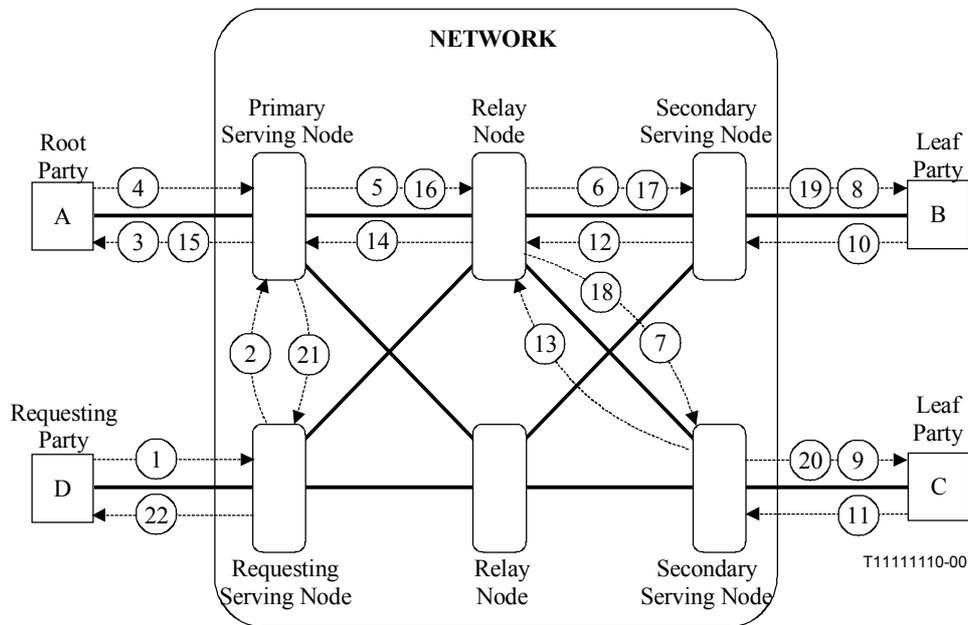
**Figure 7-8 – Point-to-multipoint Network Connection (Type 2 between A, B and C) – Third Party – With Negotiation – No Look ahead – No Notification**
