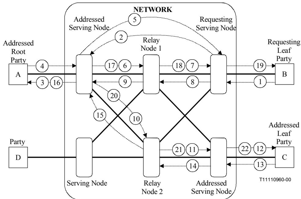
**Figure 7-2 – Three-party network connection establishment – No look-ahead – Root node branching**
