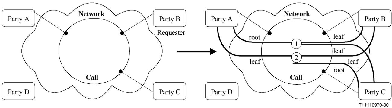
**Figure 7-3 – Call and Bearer transition diagram**
