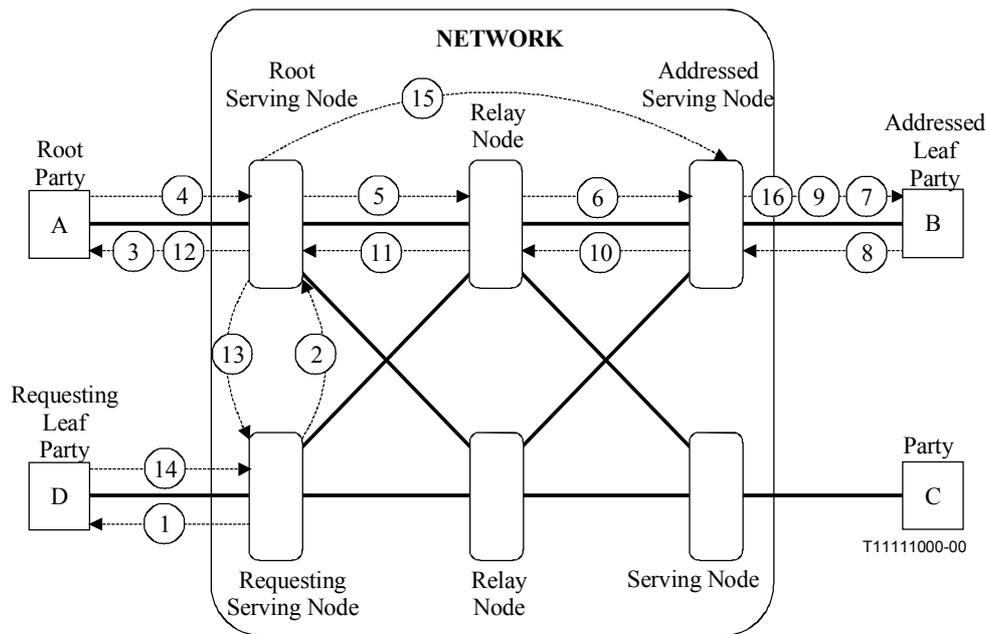
**Figure 8-2 – Attaching an existing party requested by a party which is the call owner and the leaf of the existing network connection**
