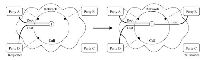
Figure 8-1 – Call and Bearer transition diagram
