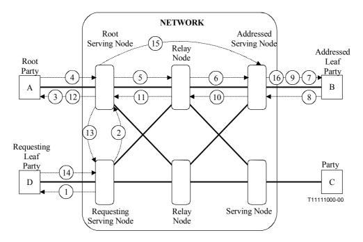
Figure 8-2 – Attaching an existing party requested by a party which is the call owner and the leaf of the existing network connection
