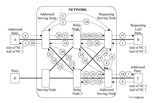
Figure 7-4 – Addition of 2 network connection establishment – No look-ahead – Root node branching – Party A is the root of network connection 1 while party C is the root of network connection 2
