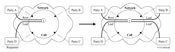
Figure 8-3 – Call and Bearer transition diagram
