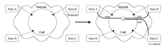
Figure 7-1 – Call and Bearer transition diagram
