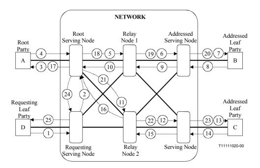
Figure 8-4 – Attachment of two existing parties requested by a party which is the call owner and the leaf of the existing network connection
