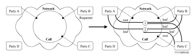
Figure 7-3 – Call and Bearer transition diagram
