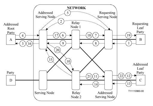
Figure 7-2 – Three-party network connection establishment – No look-ahead – Root node branching
