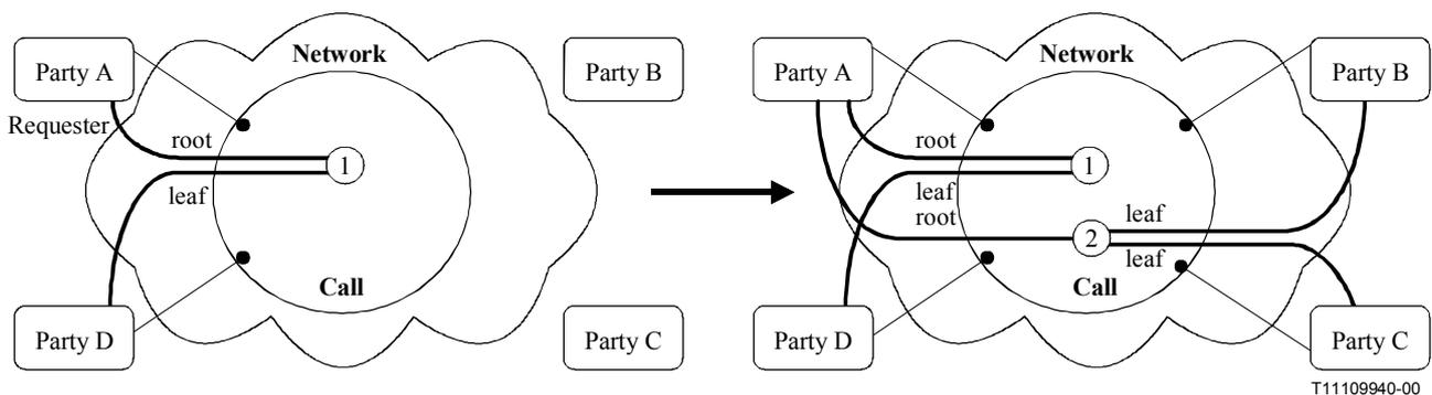
**Figure 8-7 – Call and Bearer transition diagram**
