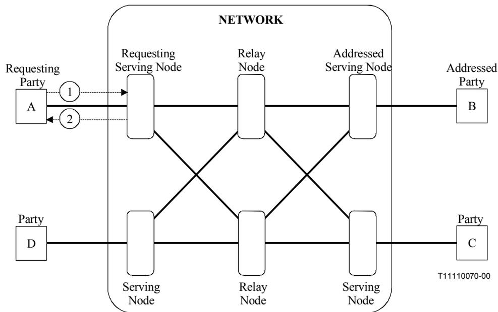
**Figure 10-2 – Release Call requested by party "A" – One network connection between parties A and the network with party A as the call and connection owner**
