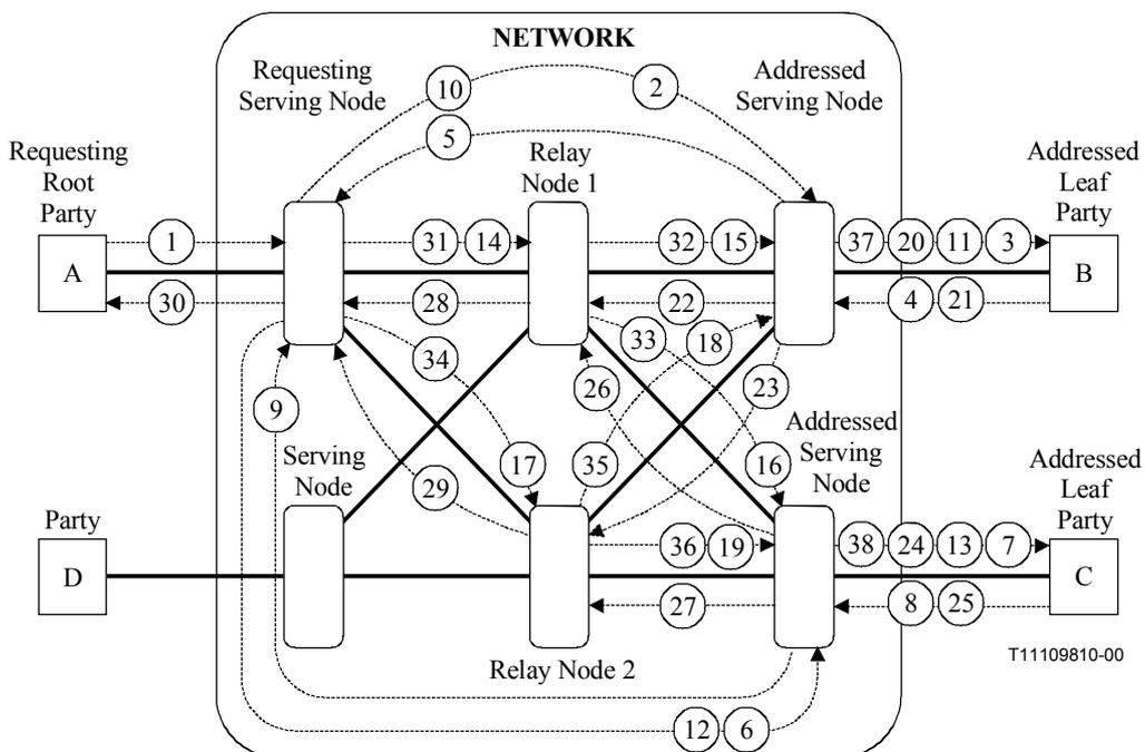
**Figure 7-12 – Three Party-two network connections call and bearer establishment (between A, B and C) – Without look-ahead**
