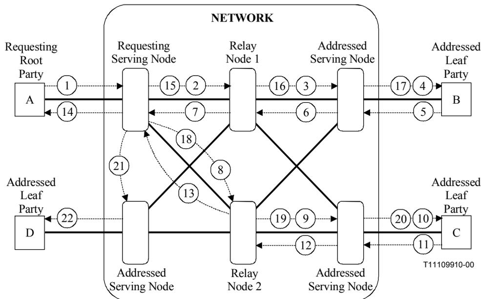
**Figure 8-4 – Add two new parties requested by a party which is the call owner and the root of the existing network connection**
