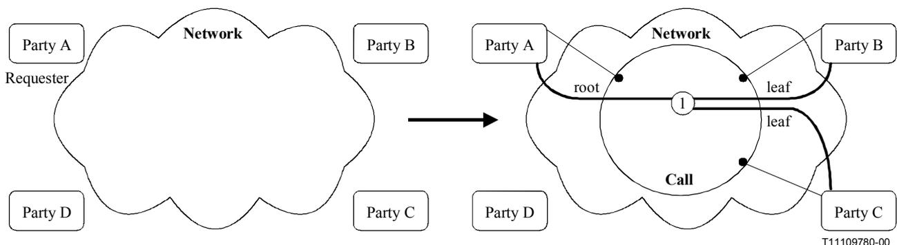
**Figure 7-9 – Call and Bearer transition diagram**
