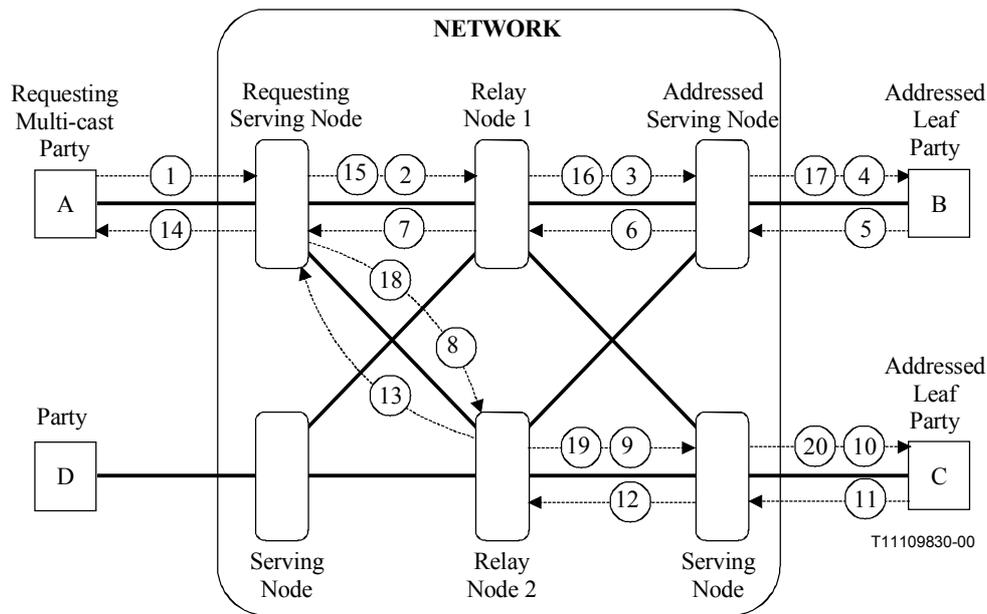
**Figure 7-14 – Mandatory multicast address call and bearer establishment**
