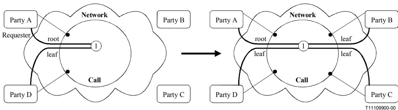
**Figure 8-3 – Call and Bearer transition diagram**
