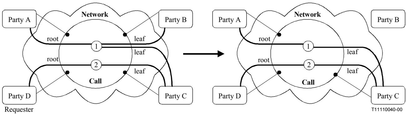
**Figure 9-9 – Call and Bearer transition diagram**
