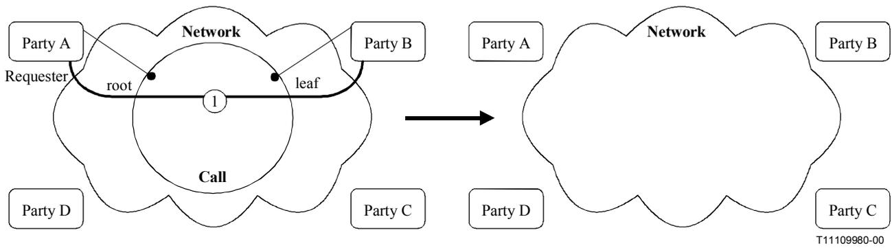
**Figure 9-3 – Call and Bearer transition diagram**
