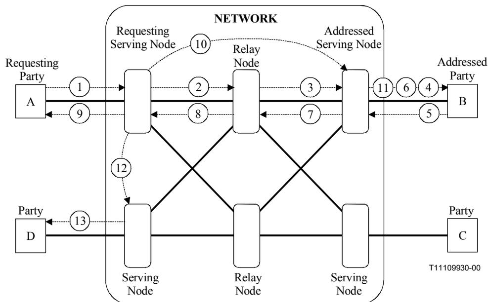
Figure 8-6 – Add one new party and a new connection requested by a party which is the call owner and will be the root of the new network connection
