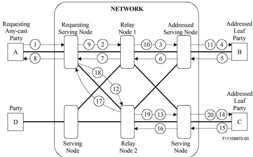
**Figure 7-18 – Any-cast address call and bearer establishment**
