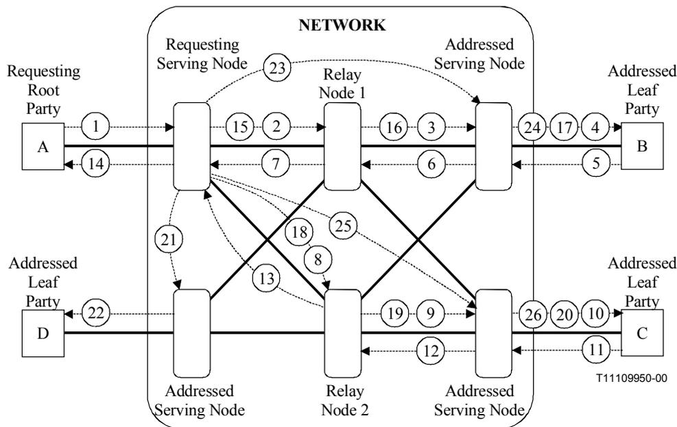
**Figure 8-8 – Add two new parties and a new connection requested by a party which is the call owner and will be the root of the new network connection**
