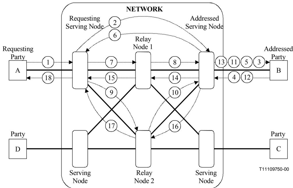
**Figure 7-6 – Two network connections (between A and B) – Without look-ahead**
