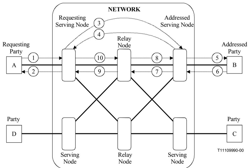
**Figure 9-4 – Release party "B" from Call requested by party "A" – One network connection between parties A and B with party A as the call and connection owner**
