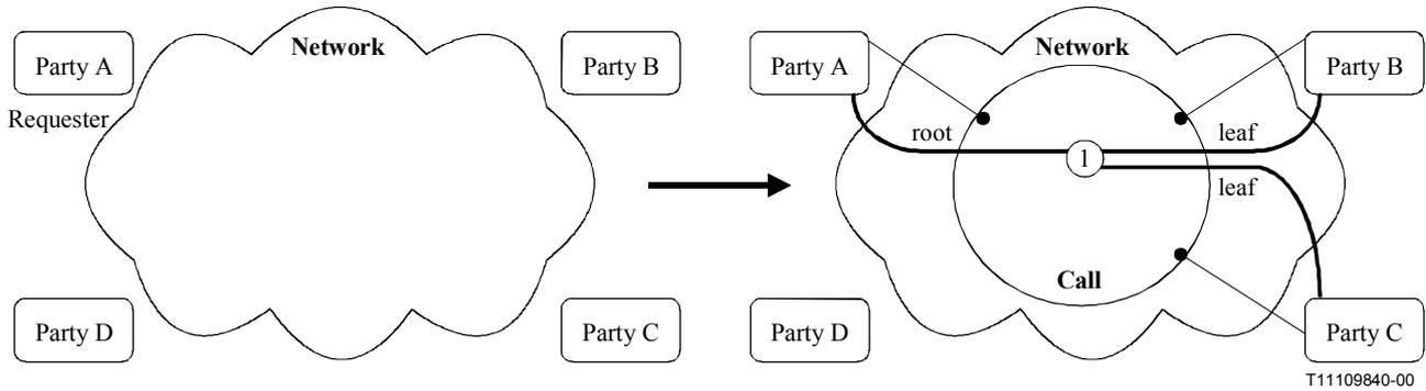
**Figure 7-15 – Call and Bearer transition diagram**
