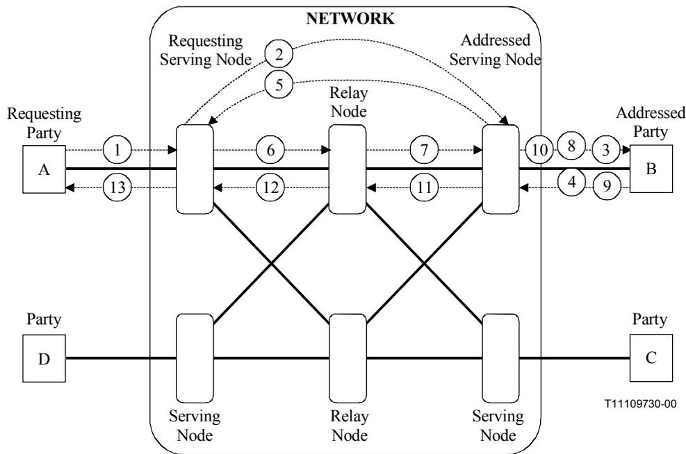
**Figure 7-4 – Single network connection (type 1 between A and B) – Look-ahead**
