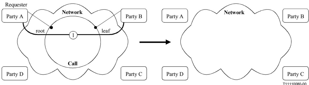
**Figure 10-3 – Call and Bearer transition diagram**
