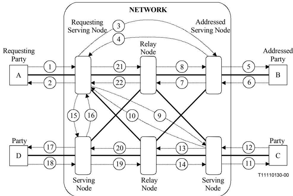
**Figure 10-8 – Release Call requested by party "A" – One network connection between parties A and B and one network connection between parties C and D with party A as the call owner**
