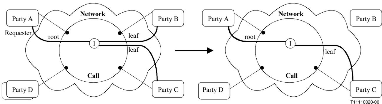
**Figure 9-7 – Call and Bearer transition diagram**
