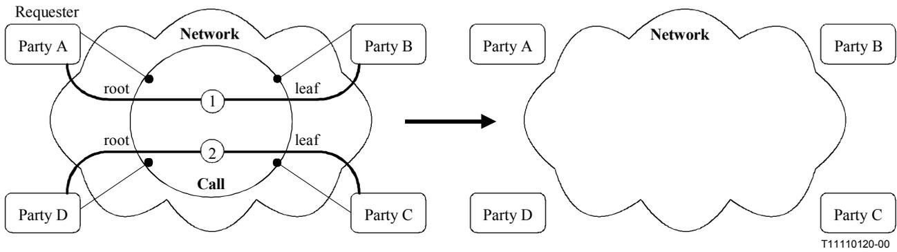
**Figure 10-7 – Call and Bearer transition diagram**
