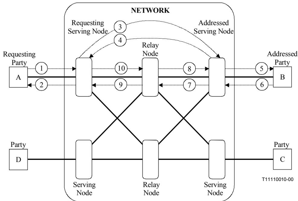
**Figure 9-6 – Release party "B" from Call requested by party "A" – One network connection between parties A and B with party A as the call and connection owner**
