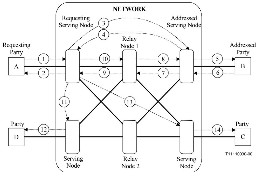
**Figure 9-8 – Release party "B" from Call requested by party "A" – One network connection between parties A, B and C, Party D is a member of the call – Party A is the call and connection owner and the root-party of the connection – Branching point occurs in the relay node 1**
