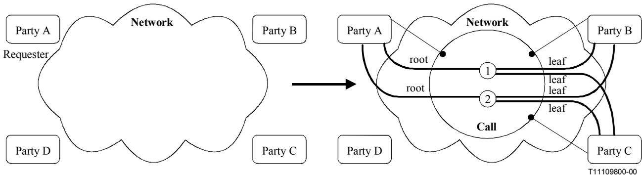
**Figure 7-11 – Call and Bearer transition diagram**
