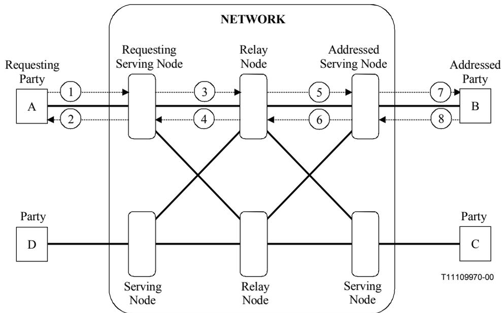
**Figure 9-2 – Release party "B" from Call requested by party "A" – One network connection between parties A and B with party A as the call and connection owner**
