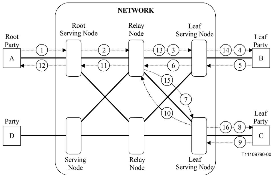
**Figure 7-10 – Three-party call and network connection establishment – No look-ahead – Relay. branch-Root)**
