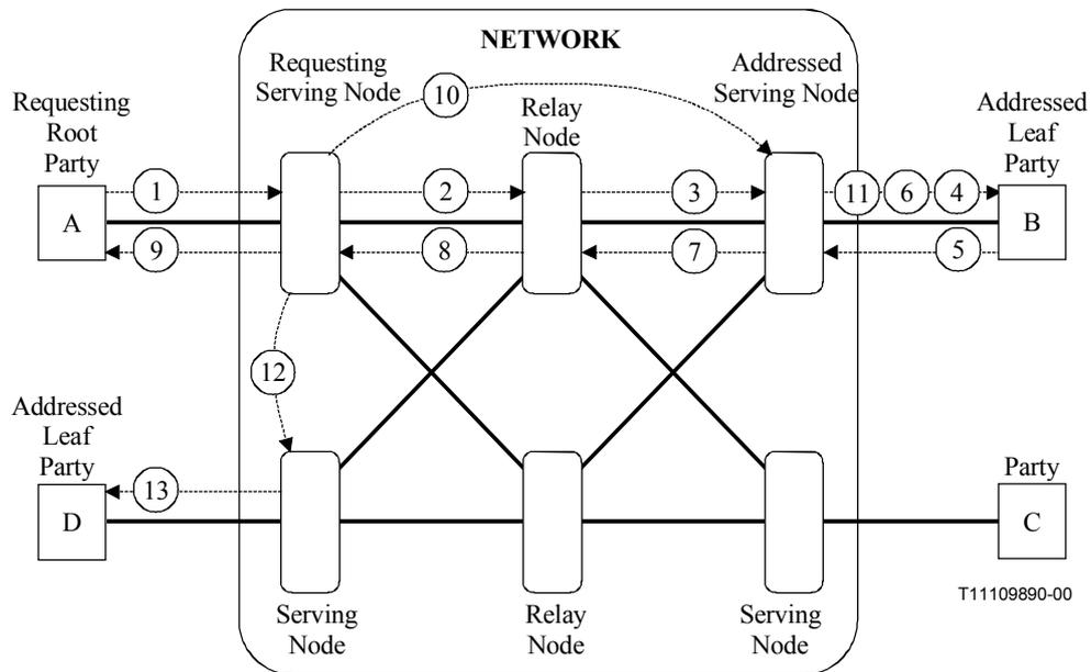
**Figure 8-2 – Add one new party requested by a party which is the call owner and the root of the existing network connection**
