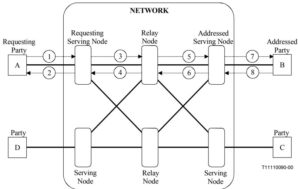
**Figure 10-4 – Release Call requested by party "A" – One network connection between parties A and B with party A as the call and connection owner**
