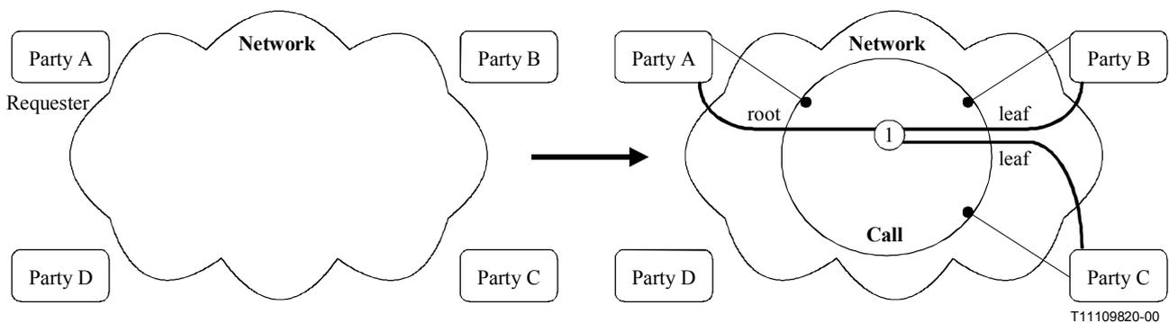
**Figure 7-13 – Call and Bearer transition diagram**
