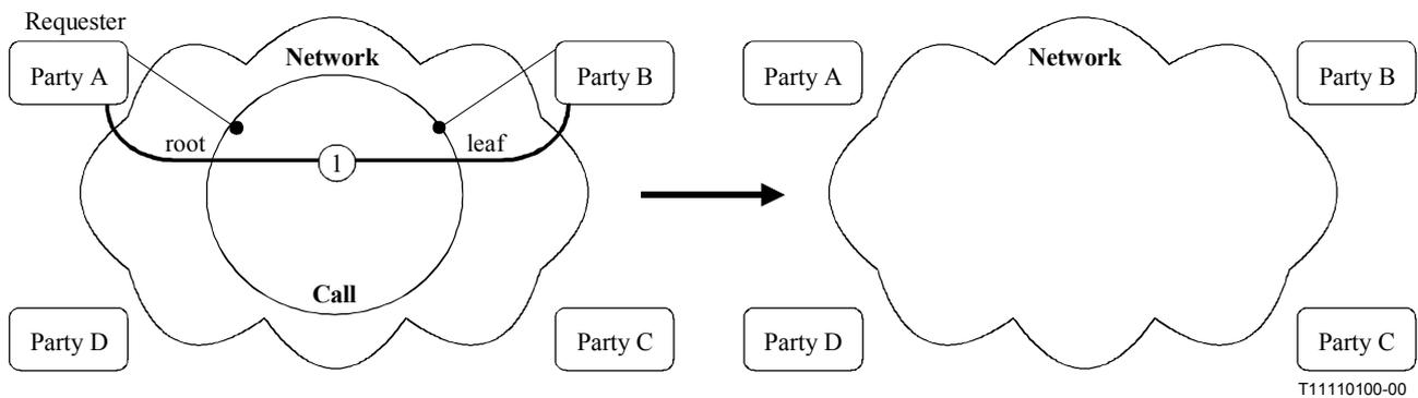
**Figure 10-5 – Call and Bearer transition diagram**
