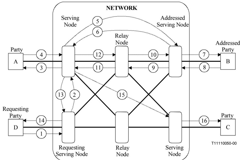
**Figure 9-10 – Release party "B" from Call requested by party "D" – Party D is a member of the call and is the party owner of party B – One network connection (1) exists between parties A, B and C – Another network connection (2) exists between parties D and C – Party A is the call and connection owner and the root-party of the connection – Branching point occurs in the relay node 1**
