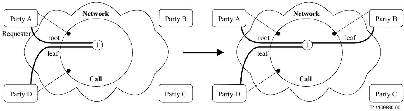
**Figure 8-1 – Call and Bearer transition diagram**
