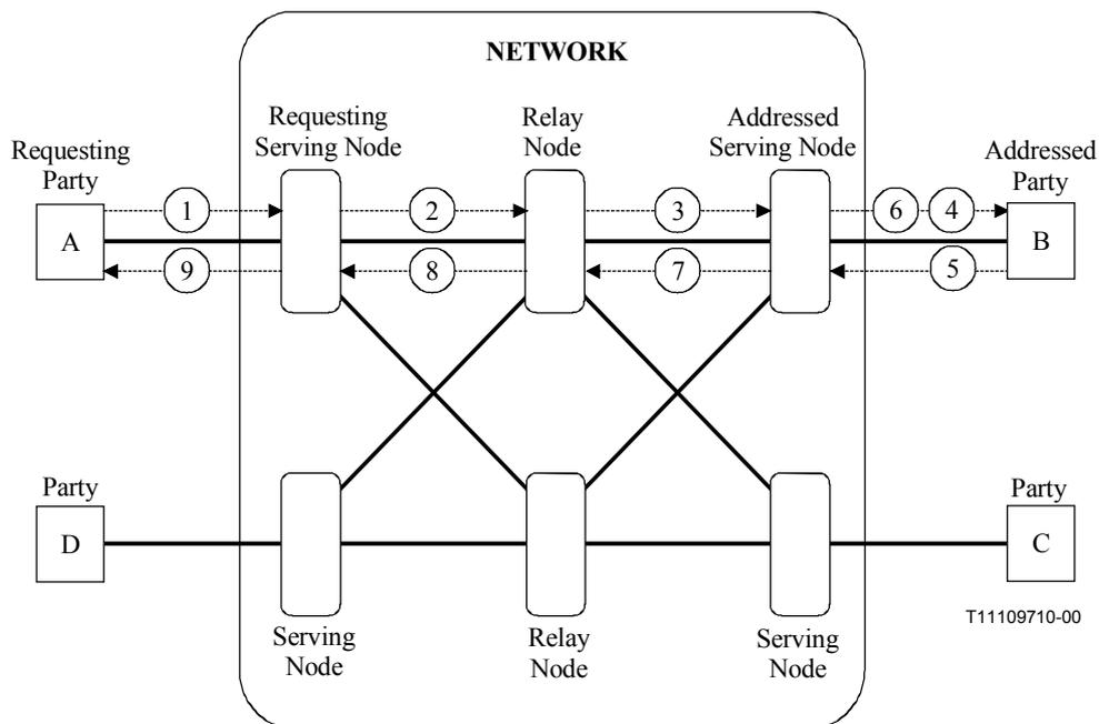
**Figure 7-2 – Single network connection (between A and B) – No look-ahead**
