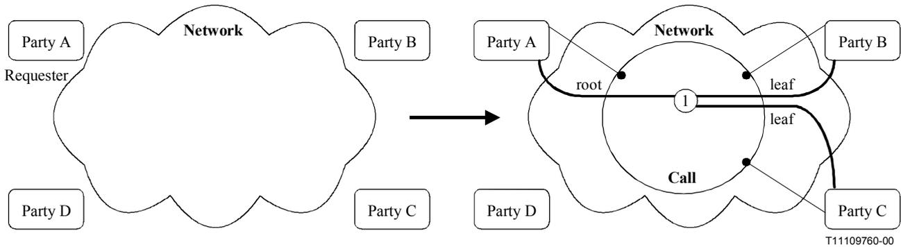
**Figure 7-7 – Call and Bearer transition diagram**
