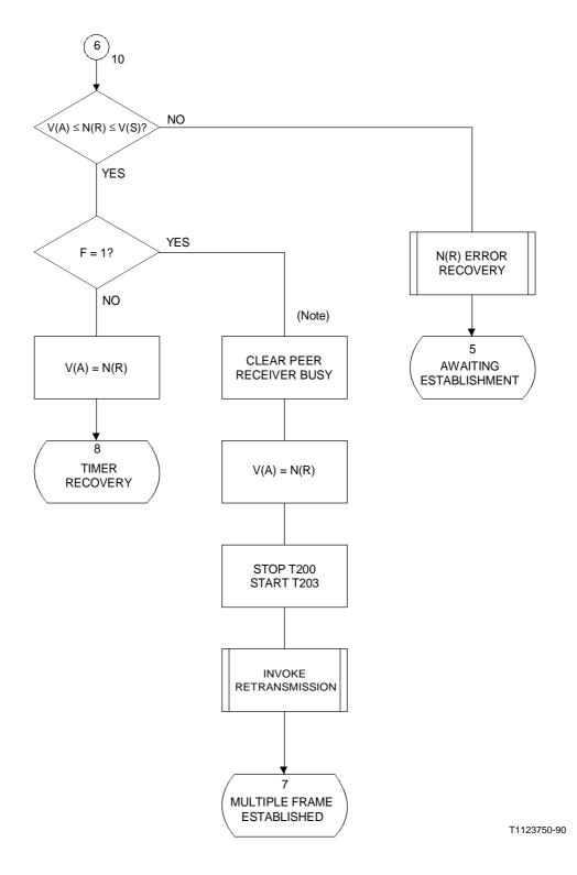
*Note* – If the peer receiver busy condition is to be maintained, the peer entity has to use an RNR response frame with the F-bit set to binary "1".
