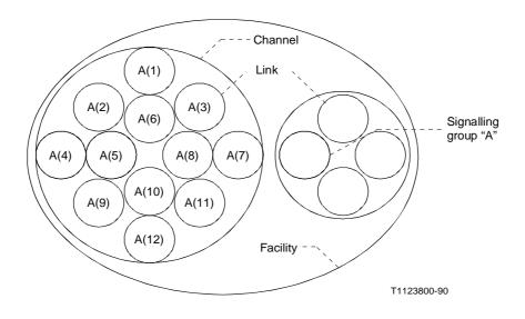
FIGURE II-3/Q.922 Channel non-associated group signalling
