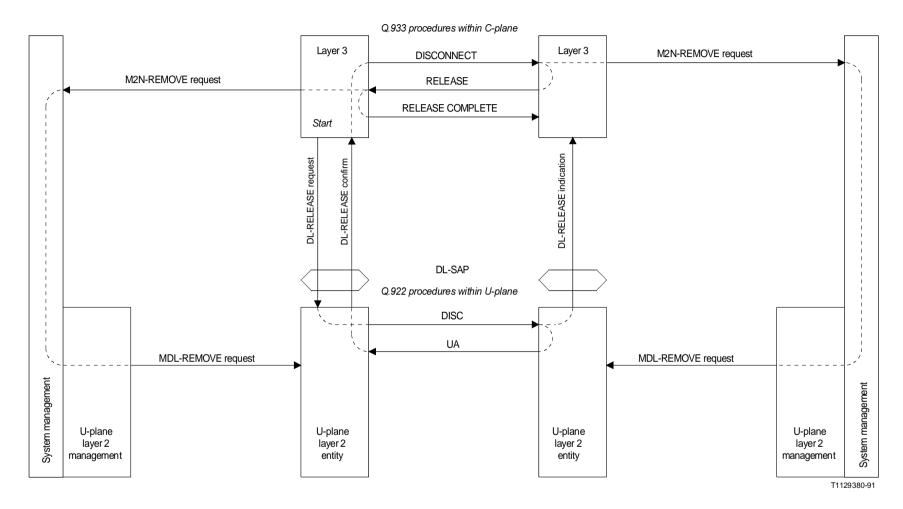
*Note* – The left side could be the network side and the right side could be the user side, or vice versa, depending upon whether the network or the user side initiates connection release.
