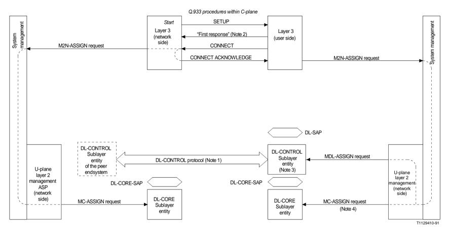
Note 1 – The DL-CONTROL protocol may be a Q.922 protocol procedure, another CCITT specified protocol, or any protocol between endsystems which, as a DL-CORE service user, is compatible with the DL-CORE sublayer services.
