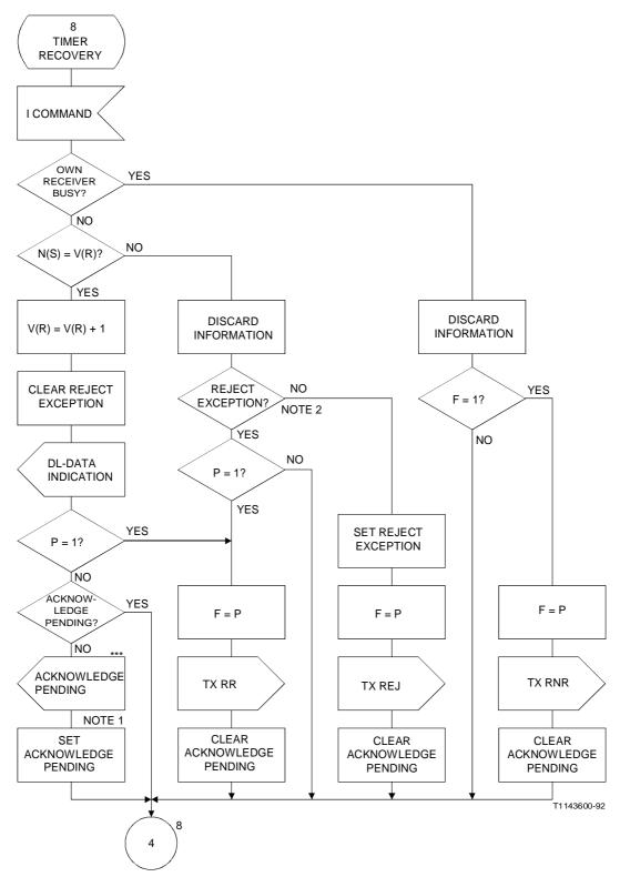
*Note 1* – Processing of acknowledge pending is described in Figure 8/Q.922 (9 of 11). *Note 2* – This SDL representation does not include the optional procedure in Appendix I of Recommendation Q.921 [2]. *Note 3* – This figure is unchanged from Recommendation Q.921 [2].
