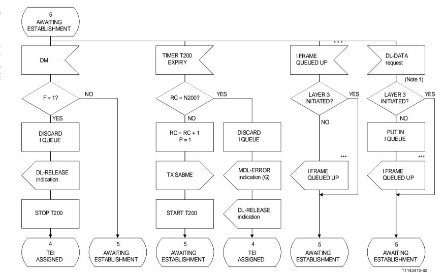
*Note 1* – Only possible in cases of layer 2 initiated re-establishment. *Note 2* – This figure is unchanged from Recommendation Q.921 [2].
