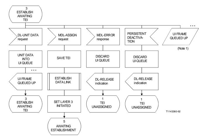
*Note 1* – Processing of UI frame queued up is described in Figure B-9/Q.922. *Note 2* – This figure is unchanged from Recommendation Q.921 [2].
