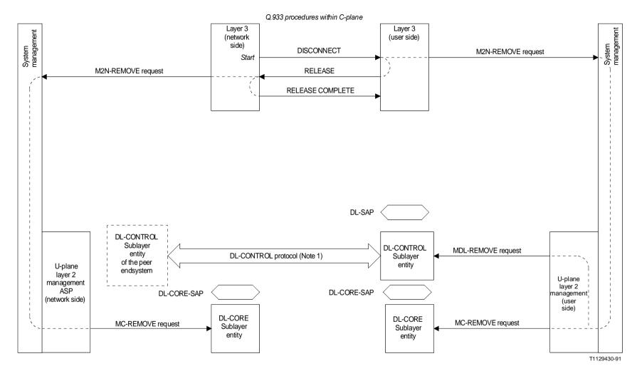
Note 1 – The DL-CONTROL protocol may be a Q.922 protocol procedure, another CCITT specified protocol, or any protocol between endsystems which, as a DL-CORE service user, is compatible with the DL-CORE sublayer services.
