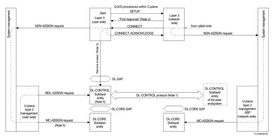
Note 1 – The DL-CONTROL protocol may be a Q.922 protocol procedure, another CCITT specified protocol, or any protocol between endsystems which, as a DL-CORE service user, is compatible with the DL-CORE sublayer services.
