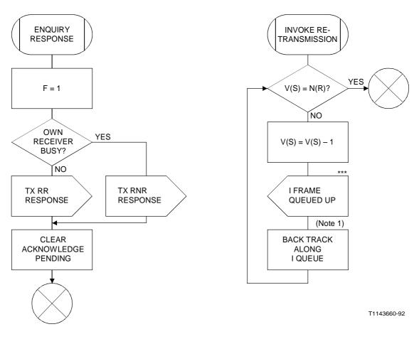
*Note 1* – The generation of the correct number of signals in order to cause the required retransmission of I frames does not alter their sequence integrity.
