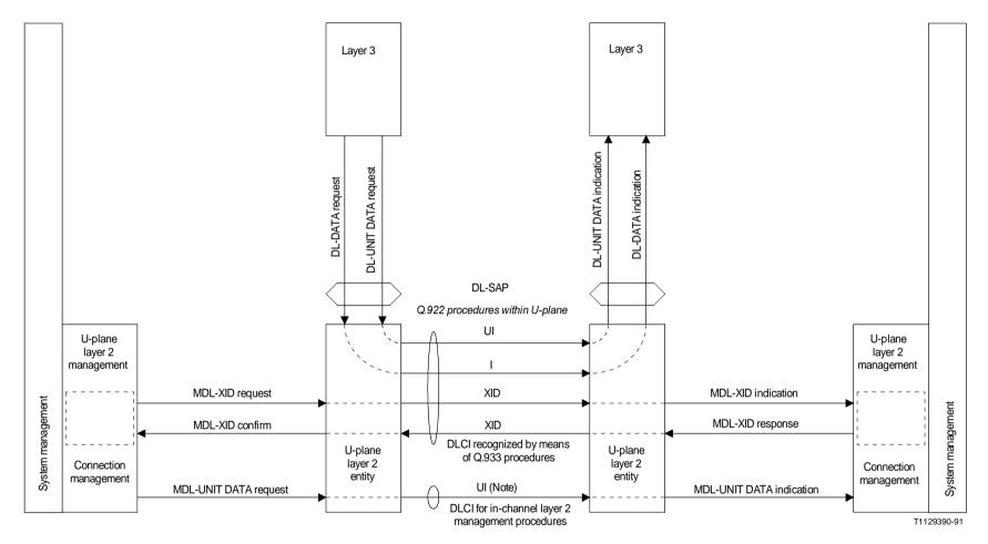
Note - Only on the link identified by the preassigned DLCI for in-channel management.
