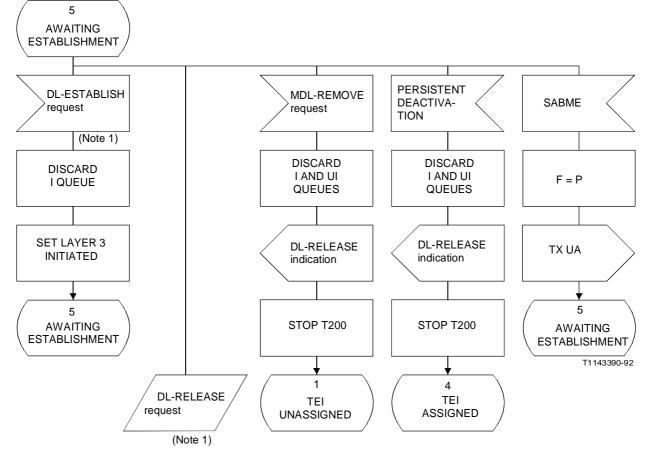
Note 1 – Only possible in cases of layer 2 initiated re-establishment. Note 2 – This figure is unchanged from Recommendation Q.921 [2].
