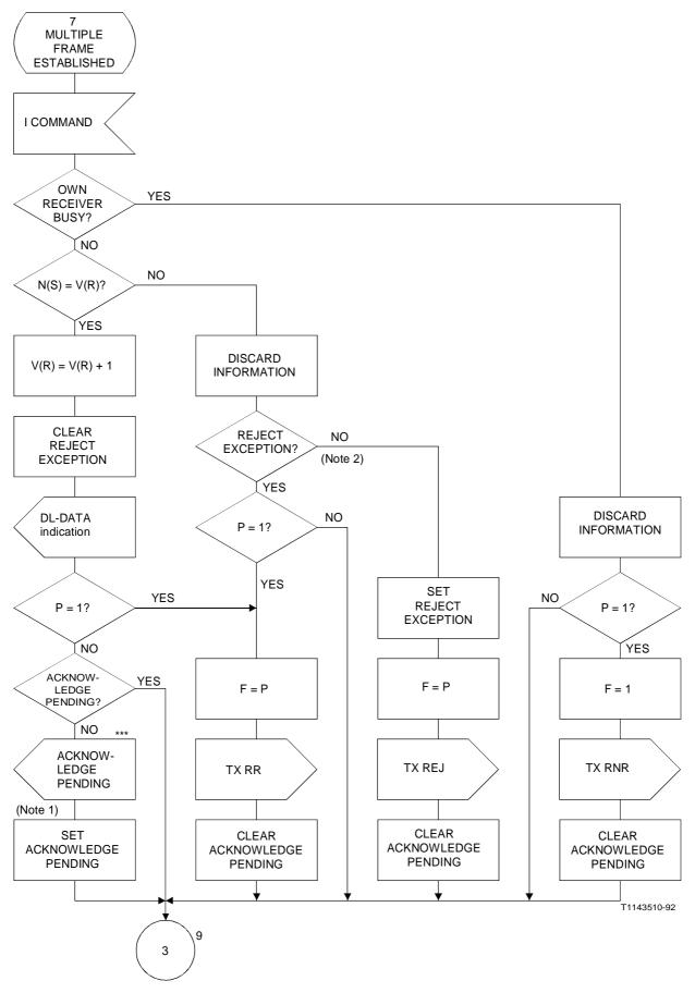
Note 1 – Processing of acknowledge pending is described in Figure B-7/Q.922 (sheet 10 of 12).
