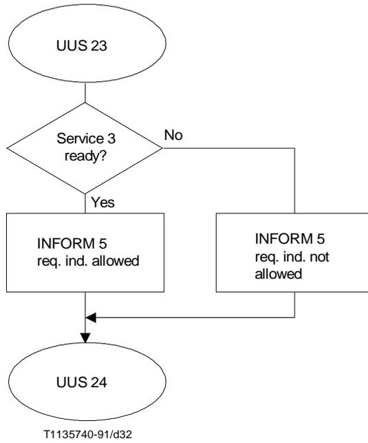
NOTE – UUS 23 and UUS 24 break the basic call between connectors S2/25, and S2/26.
