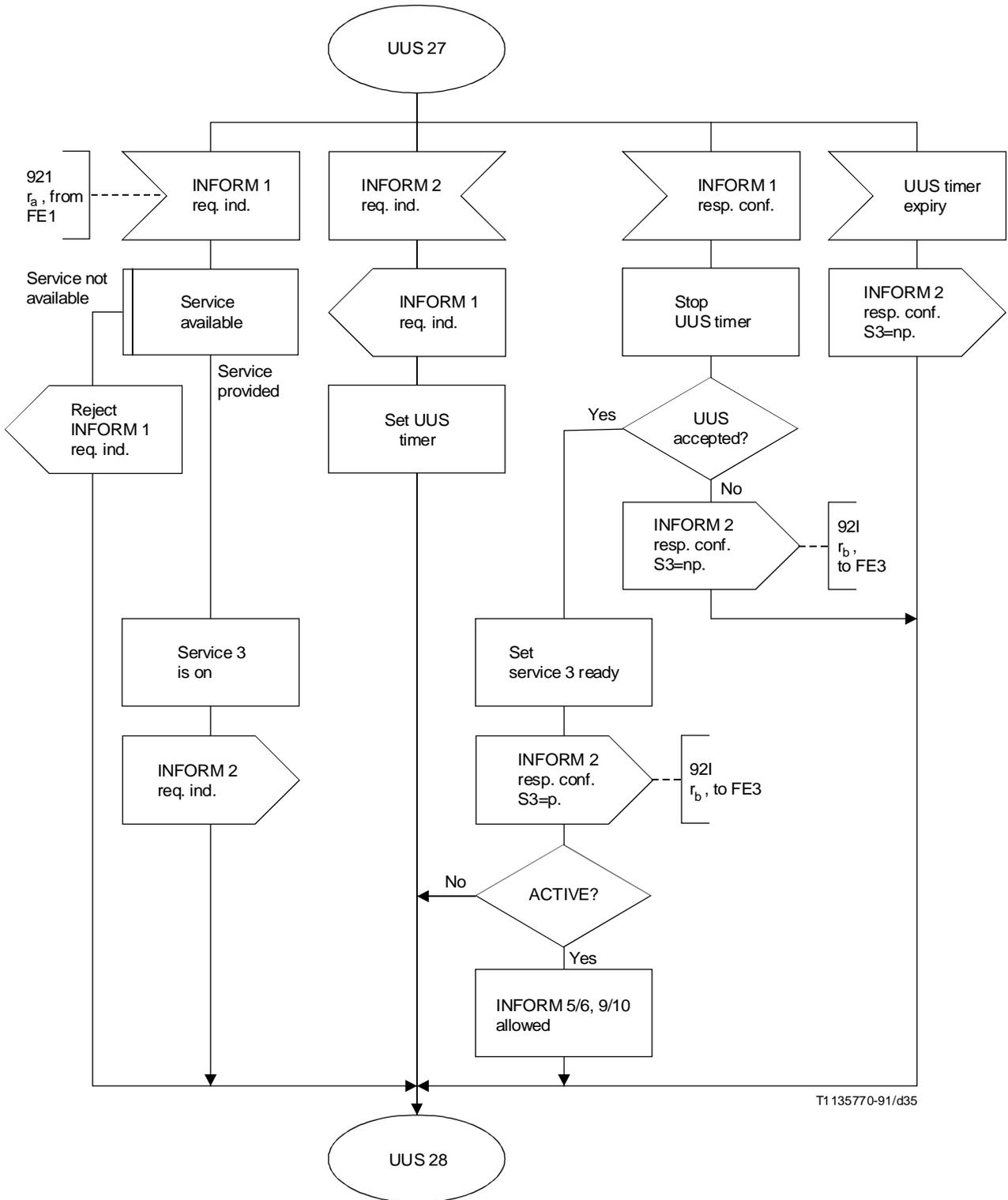
NOTE – UUS 27 and UUS 28 break the basic call between connectors S2/19 and S2/20, between connectors S2/UUS 27b and S2/UUS 28b.
