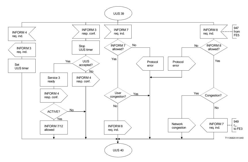
NOTE - UUS 39 and UUS 40 break the basic call between connectors S4/UUS39 and S4/UUS 40.
