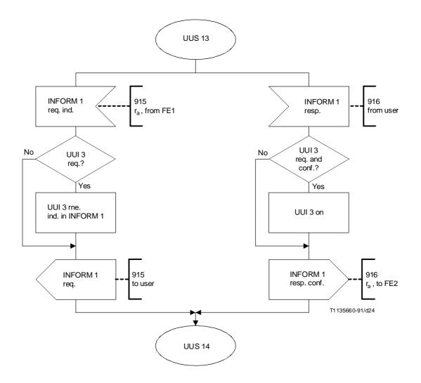
NOTE - UUS 13 and UUS 14 break the basic call between connectors S1/UUS 13 and S1/UUS 14.
