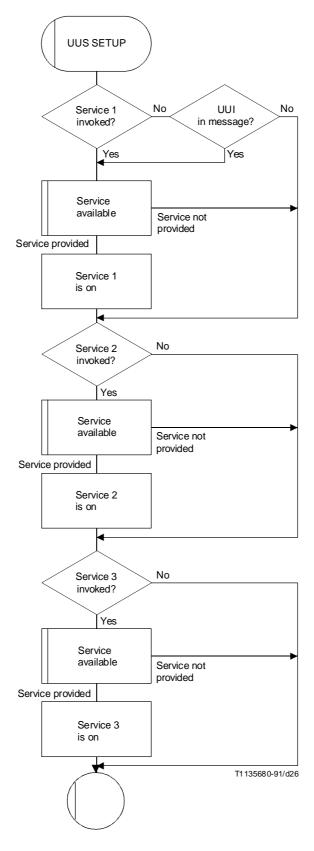
FIGURE 1-19/Q.87 Macrodefinition UUS SETUP, r1-r1
