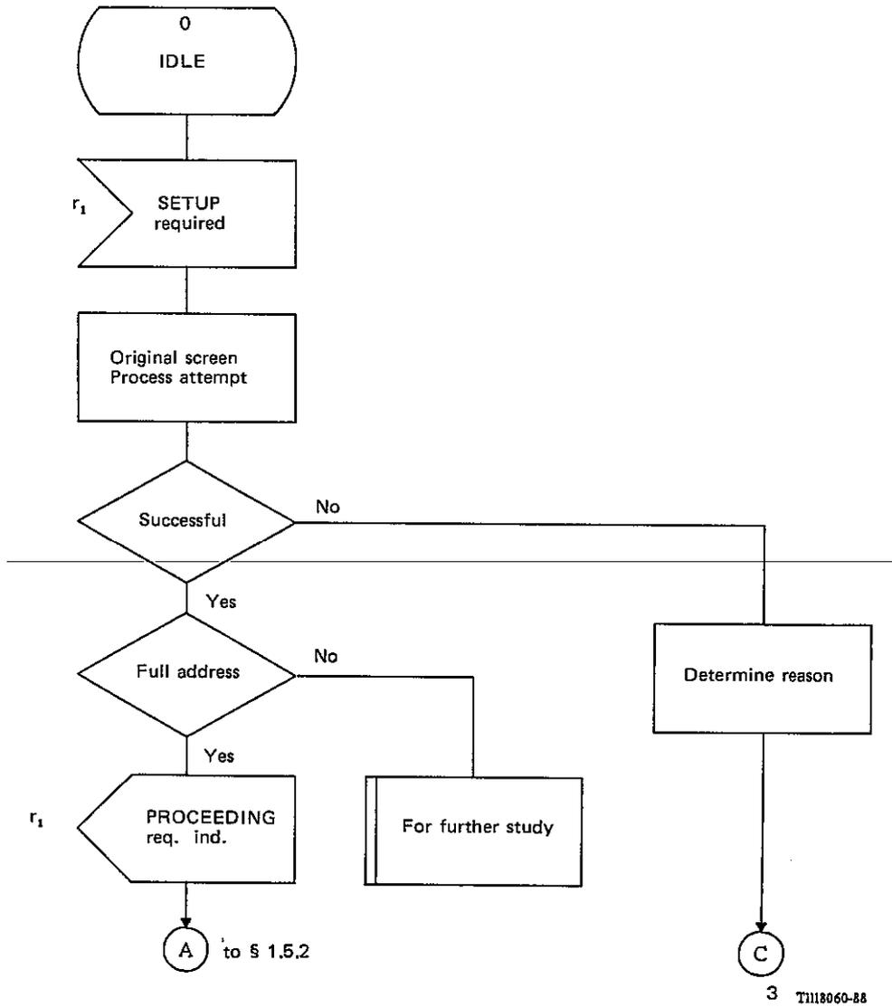
*Note* — If cause of call failure is to be conveyed by in-band tones, a B Channel must be established.
