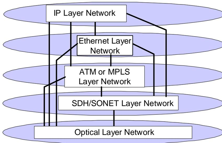
**Figure 5-3 – Network layering example**
