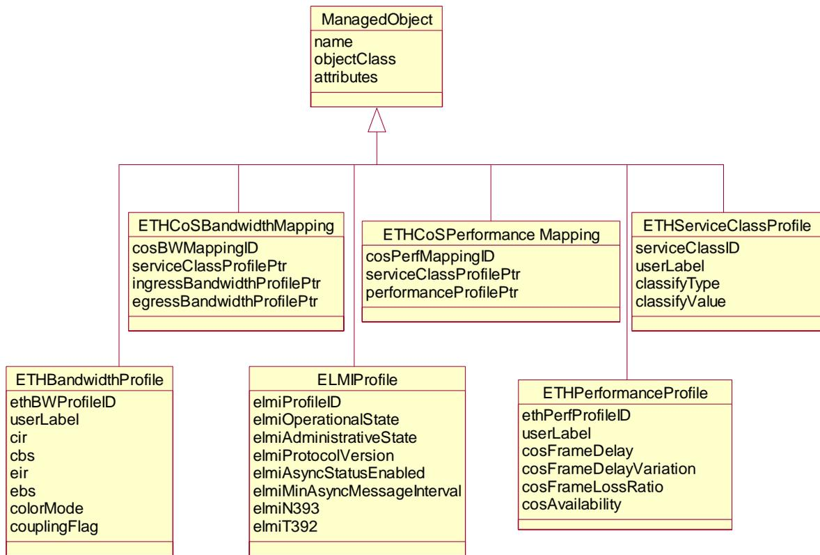
**Figure 7-3 – Inheritance diagram of Ethernet managed entities: Reference data**
