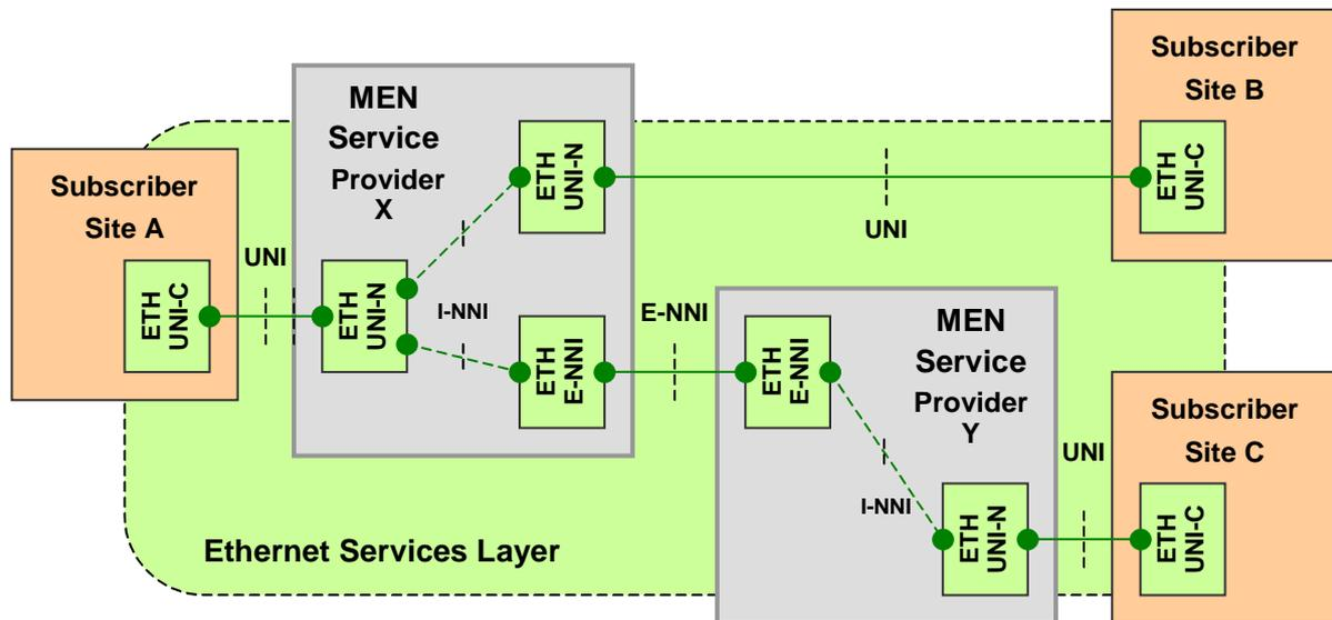
Figure 5-2 – ETH layer interfaces and reference points
