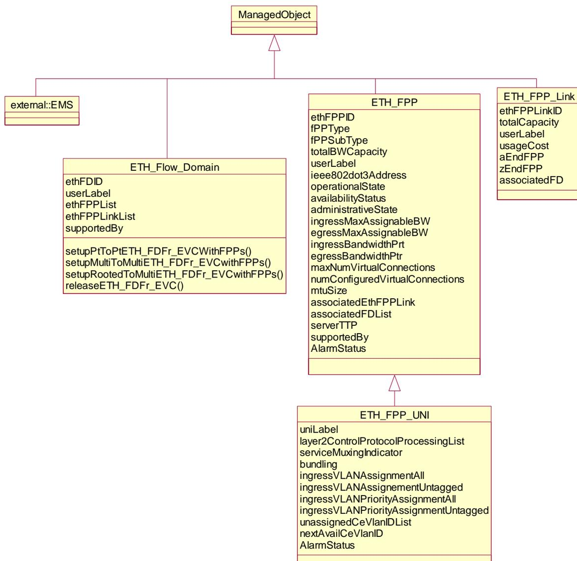
Figure 7-1 – Inheritance diagram of Ethernet managed entities: Topology view
