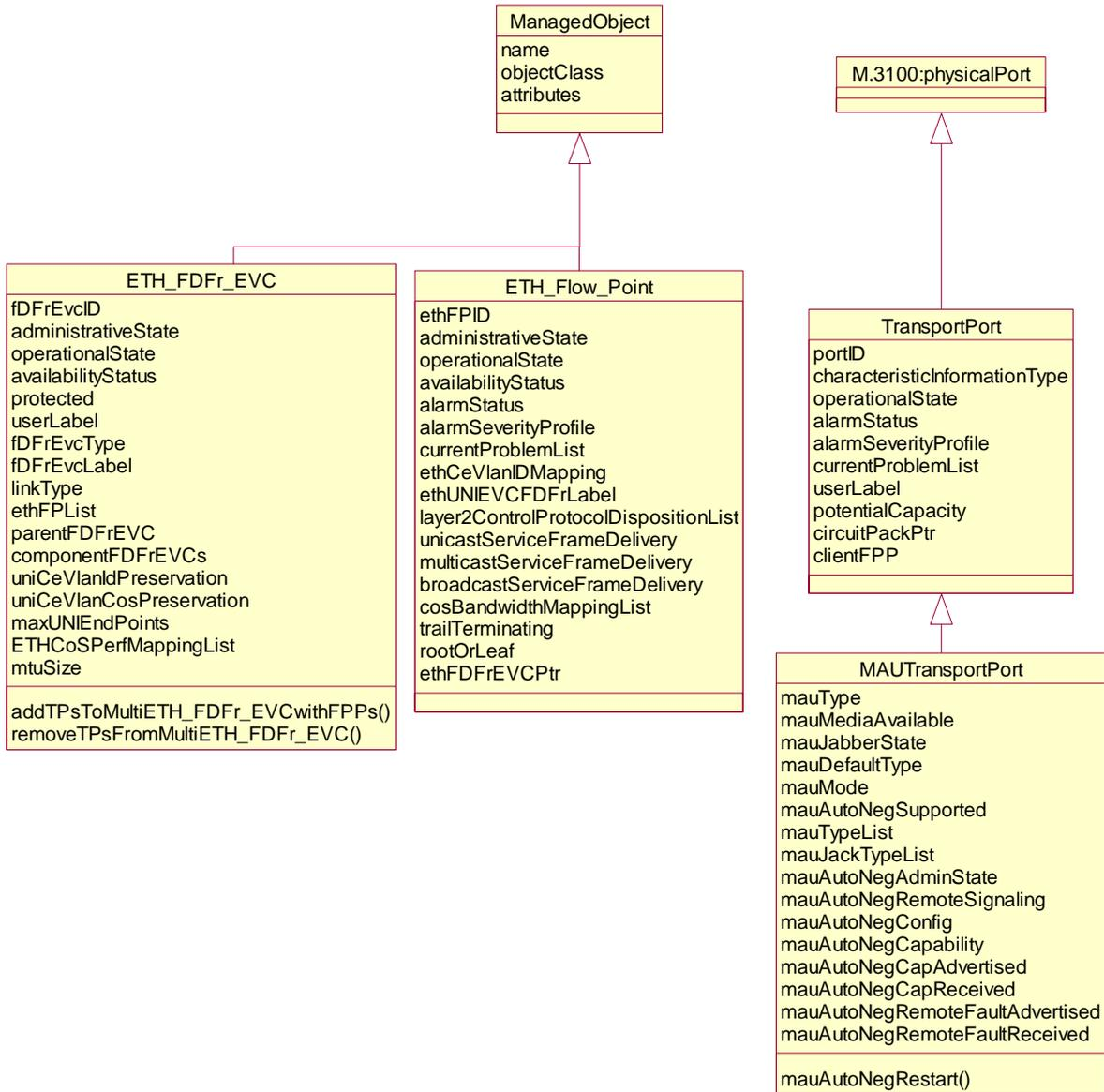
**Figure 7-2 – Inheritance diagram of Ethernet managed entities: Connectivity view**
