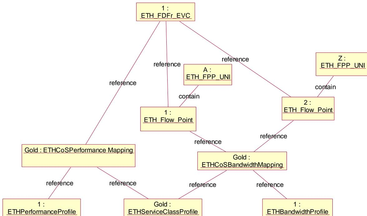
Figure II.1 – Example in object diagram
