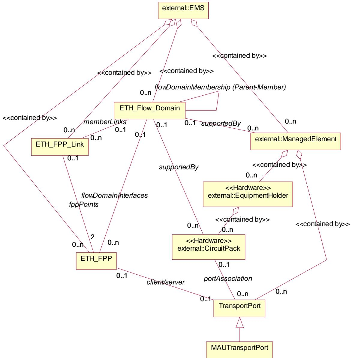
Figure 7-4 – Relationship diagram of Ethernet network view and equipment related
