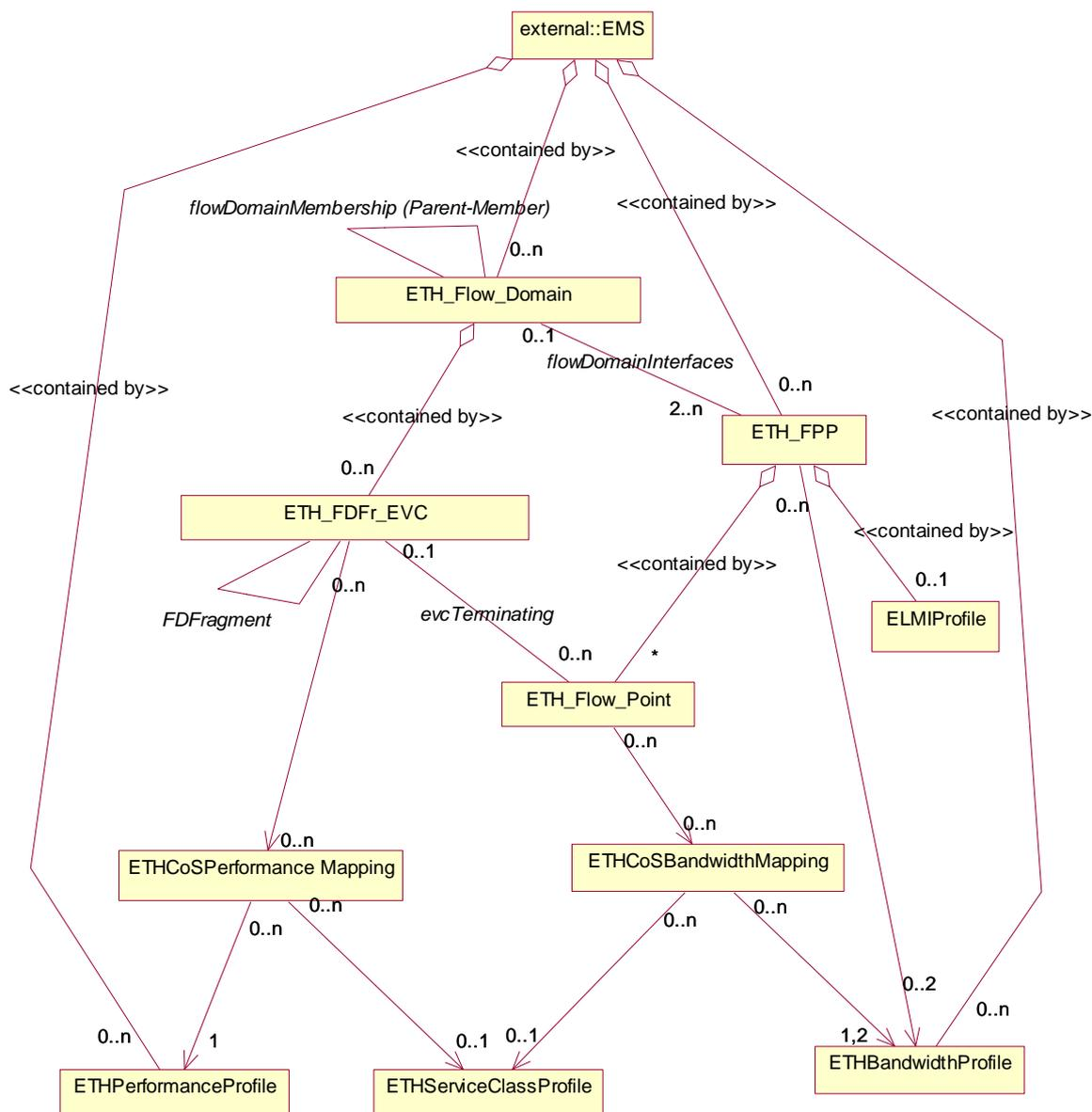
**Figure 7-5 – Relationship diagram of Ethernet service configuration managed Entities**
