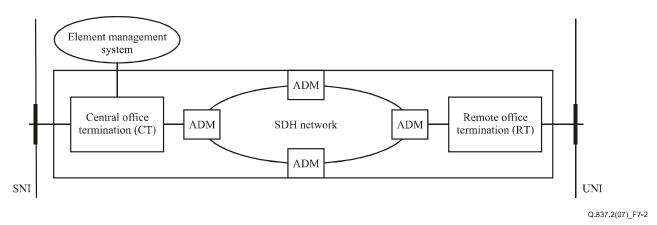
Figure 7-2 – SDH-DLC system architecture
