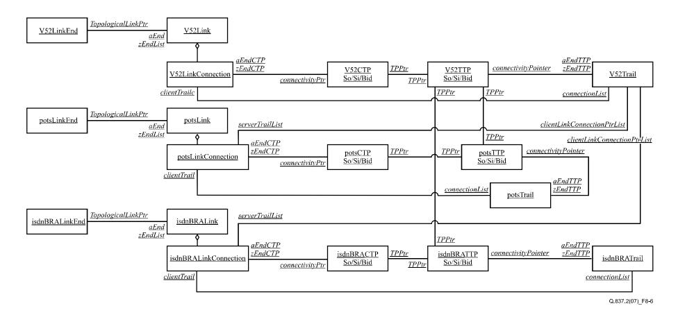
Figure 8-6 – E-R diagram of configuration management – V5.2 layer network managed entities
