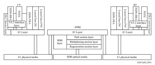
Figure 6-2 – Network layering of SDH-DLC
