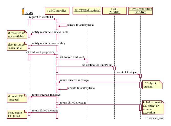
Figure 8-15 – Create SDH cross-connection sequence diagram
