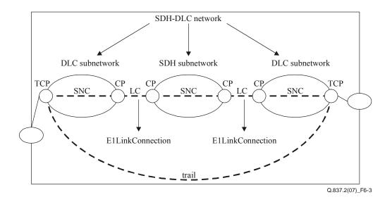
Figure 6-3 – Partitioning SDH-DLC subnetwork
