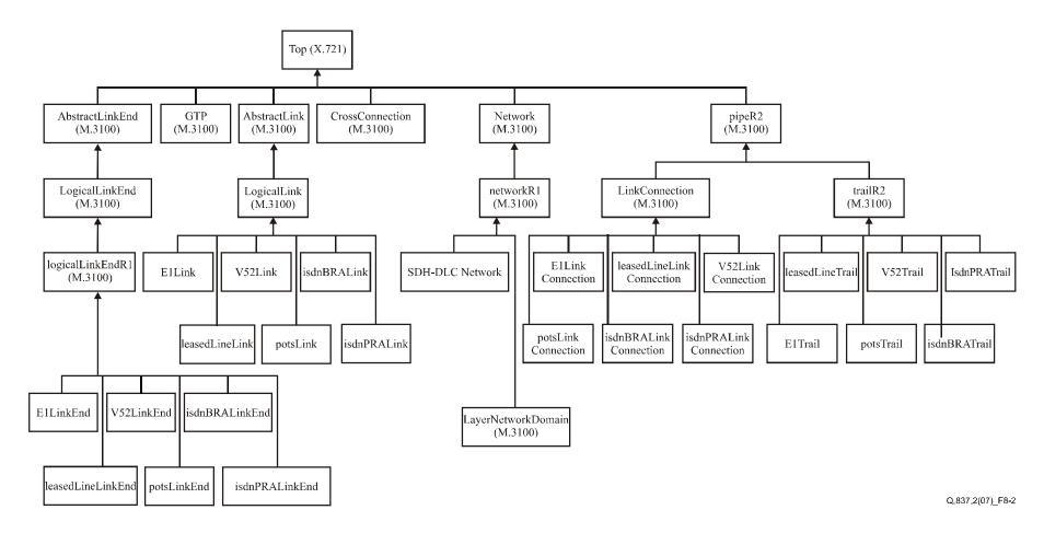
Figure 8-2 – Inheritance diagram for network view
