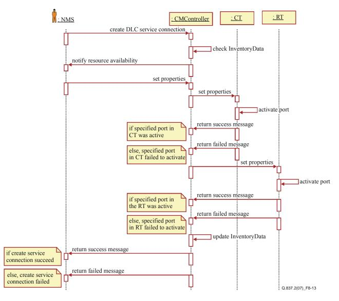
Figure 8-13 – Create DLC service connection sequence diagram
