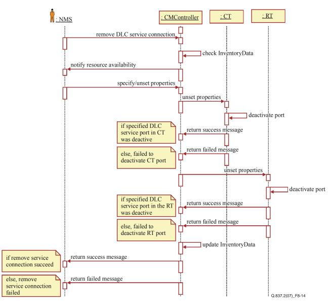
Figure 8-14 – Remove DLC service connection sequence diagram
