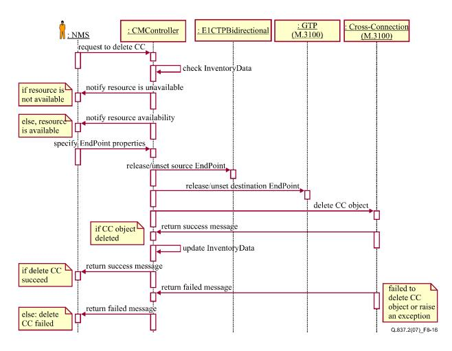
Figure 8-16 – Remove SDH cross-connection sequence diagram
