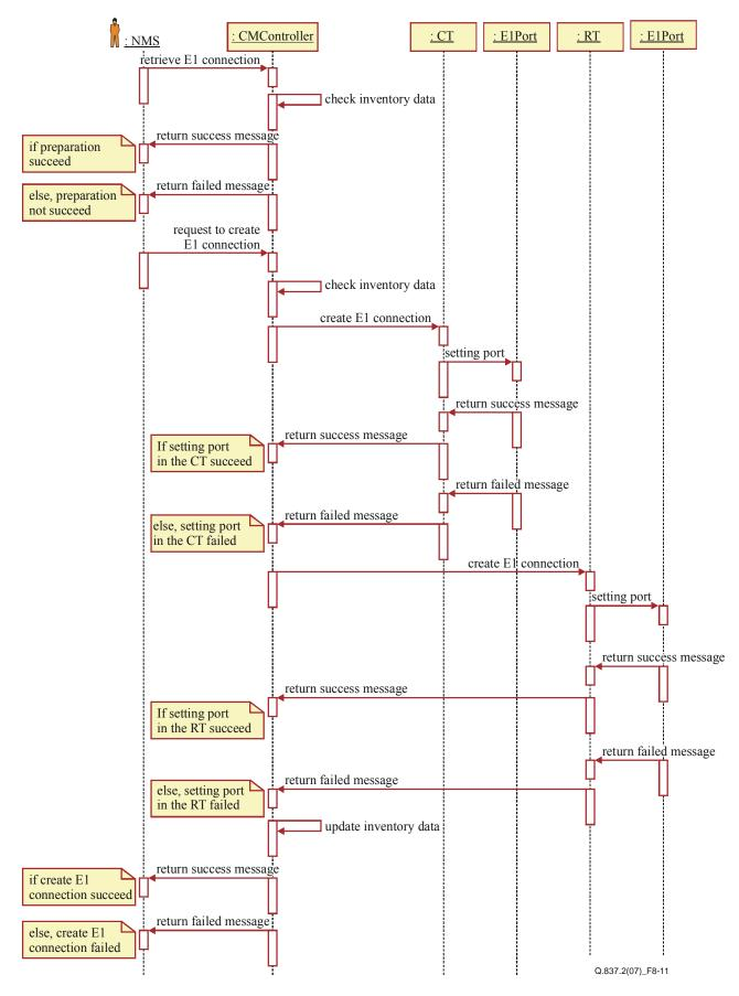
Figure 8-11 – Create E1 connection sequence diagram
