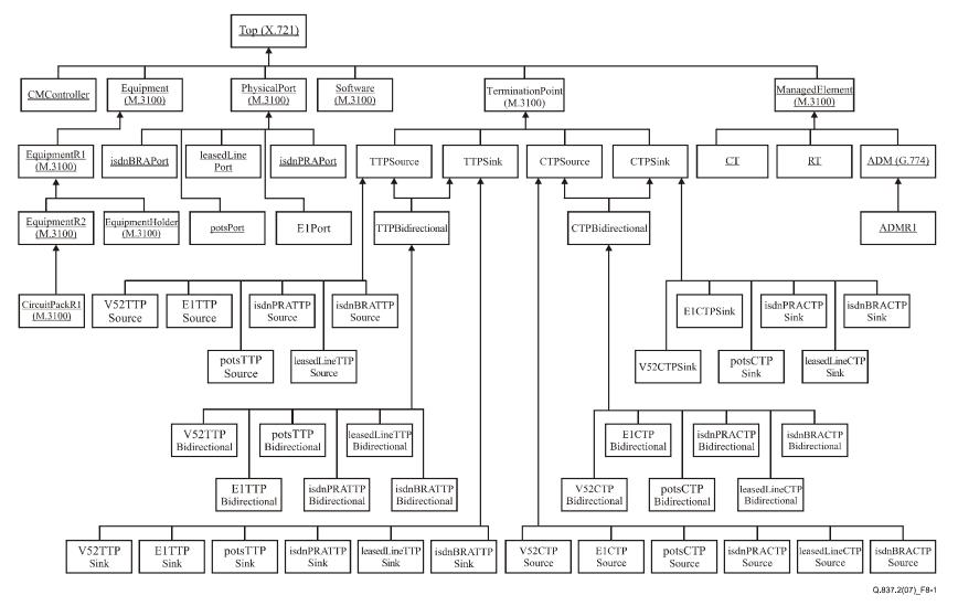
Figure 8-1 – Inheritance diagram for network element view
