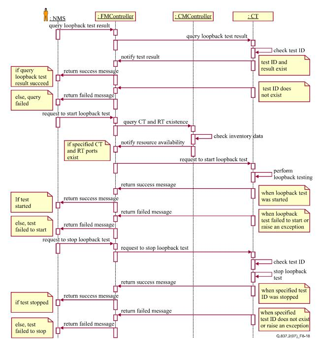
Figure 8-18 – DLC loopback test sequence diagram
