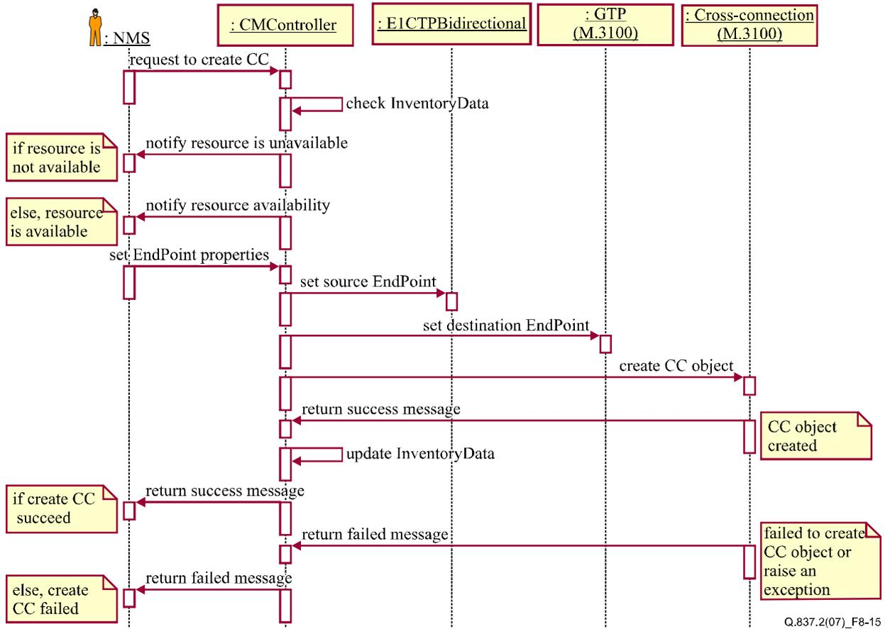
Figure 8-15 – Create SDH cross-connection sequence diagram
