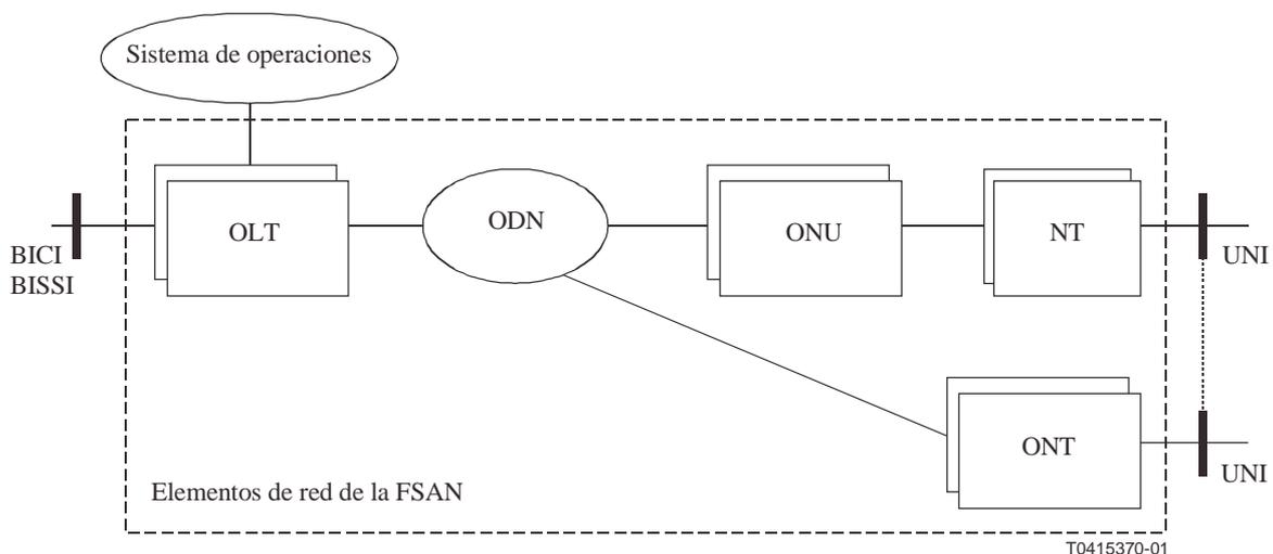
**Figura 1/Q.834.1 – Elementos de red FSAN**
