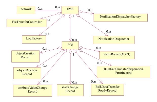
Figure 7-2.1 – Containment diagram of common management with EMS
