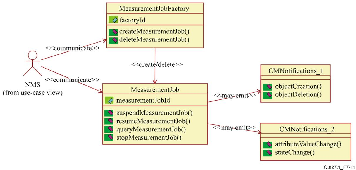
**Figure 7-11/Q.827.1 – Class diagram of measurementjob**
