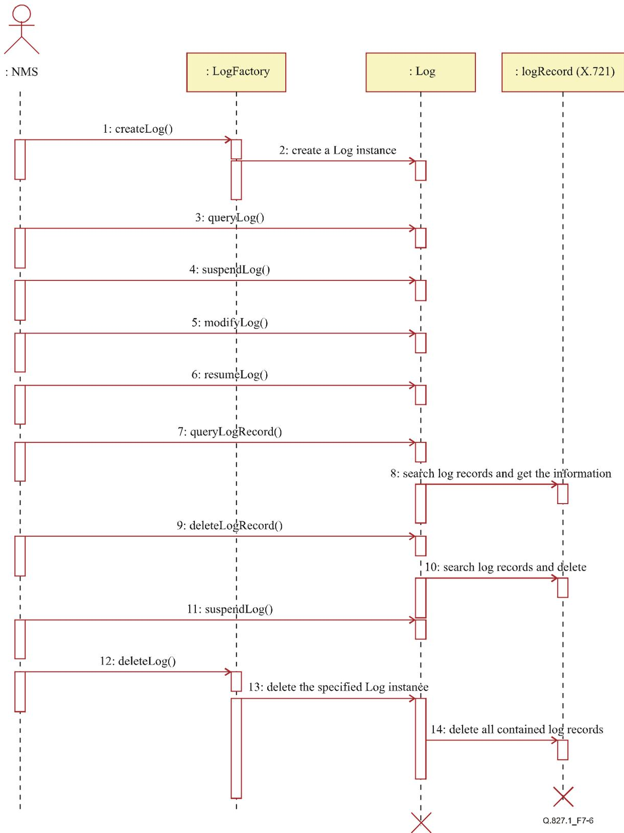
Figure 7-6/Q.827.1 – Sequence diagram of Log management functions
