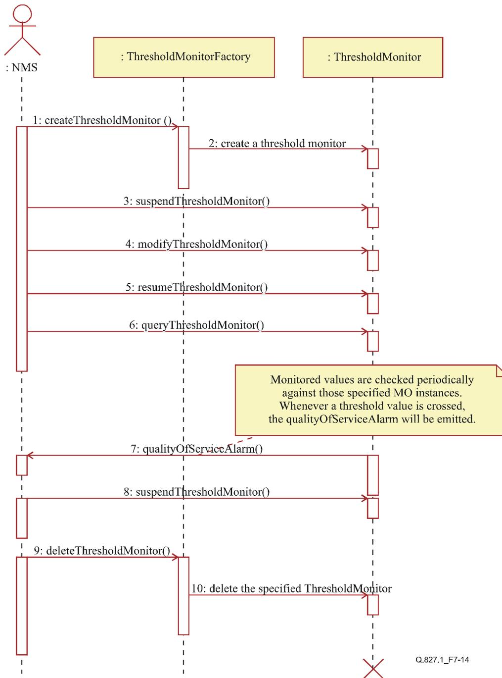
**Figure 7-14/Q.827.1 – Sequence diagram of performance threshold management**
