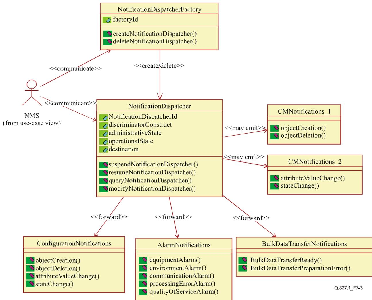
Figure 7-3/Q.827.1 – Class diagram of notification dispatcher
