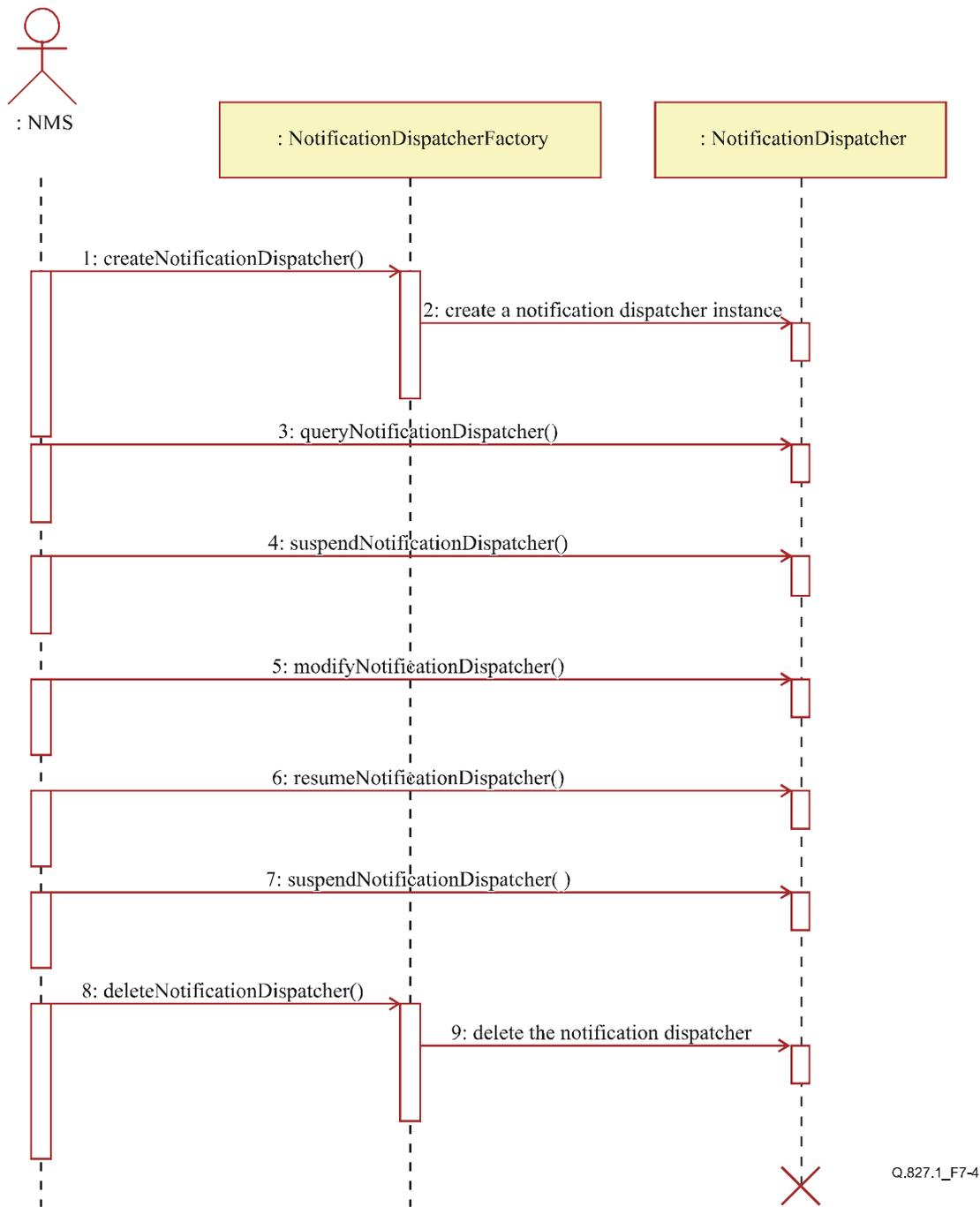
**Figure 7-4/Q.827.1 – Sequence diagram of notification dispatcher management functions**
