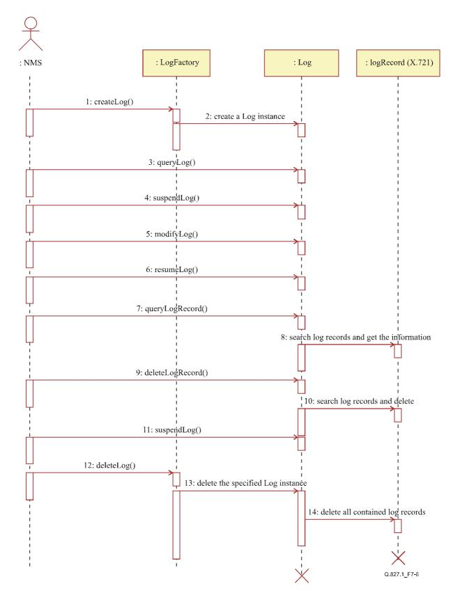
Figure 7-6/Q.827.1 – Sequence diagram of Log management functions
