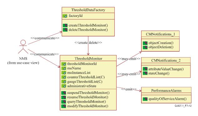
Figure 7-12/Q.827.1 – Class diagram of ThresholdMonitor
