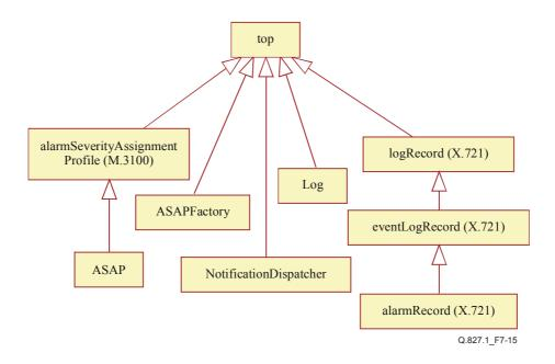
Figure 7-15/Q.827.1 – Inheritance diagram of the fault management
