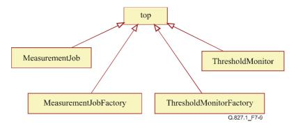
Figure 7-9/Q.827.1 – Inheritance diagram of performance management
