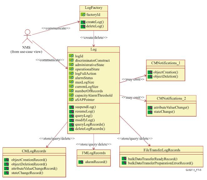
Figure 7-5/Q.827.1 – Class diagram of log
