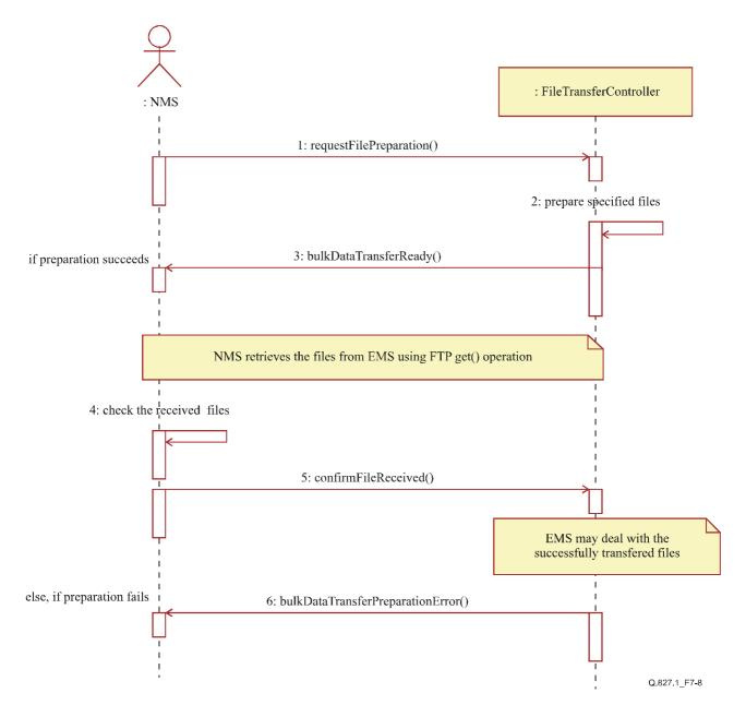
Figure 7-8/Q.827.1 – Sequence diagram of bulk data transfer control
