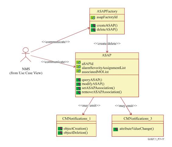
Figure 7-17/Q.827.1 – Class diagram of ASAP
