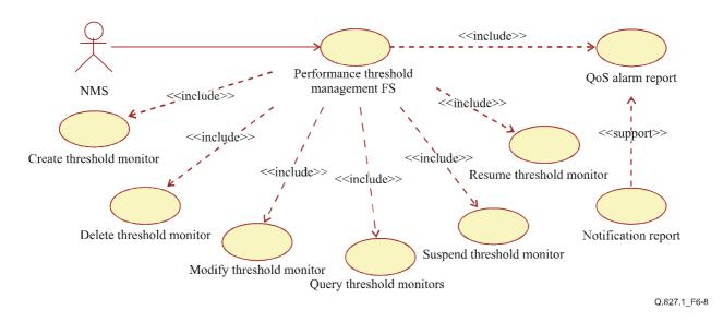
Figure 6-8/Q.827.1 – Performance threshold management function set
