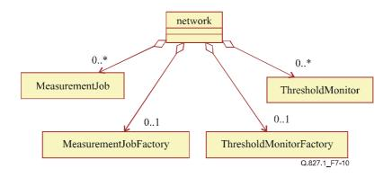
Figure 7-10/Q.827.1 – Containment diagram of performance management
