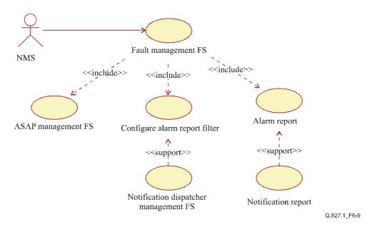
Figure 6-9/Q.827.1 – Fault management function set
