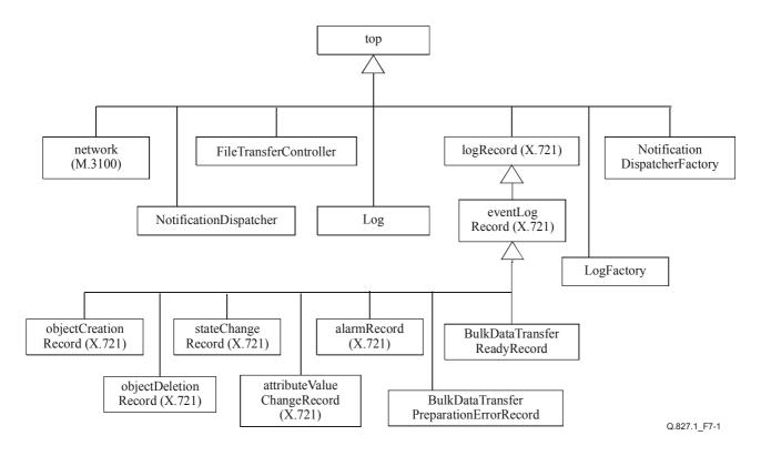
Figure 7-1/Q.827.1 – Inheritance diagram of common management
