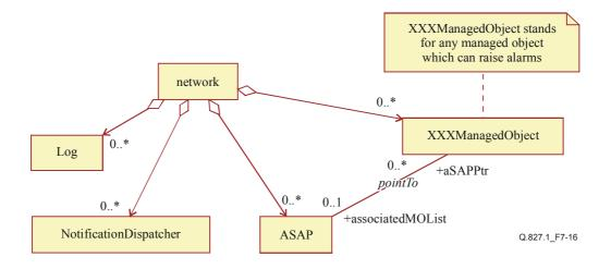
Figure 7-16/Q.827.1 – Entities relationship diagram of fault management
