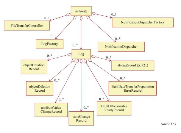
Figure 7-2/Q.827.1 – Containment diagram of common management
