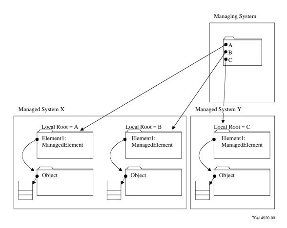
Figure 4/Q.816 – Moving a local root naming context and contained objects
