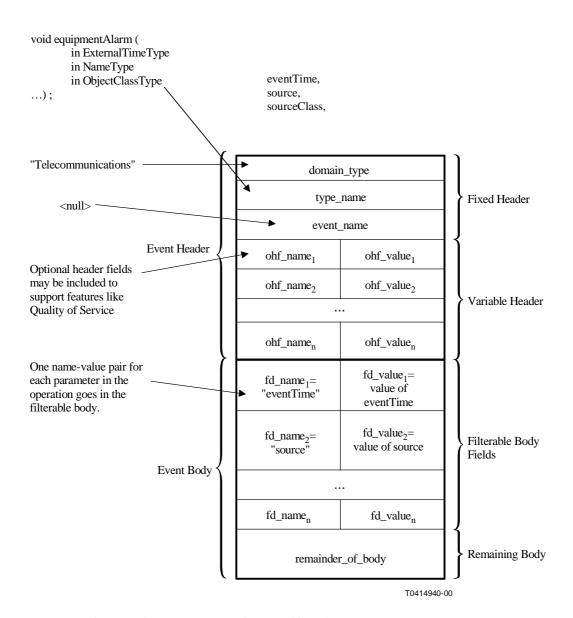
Figure 6/Q.816 – Mapping notifications to structured events
