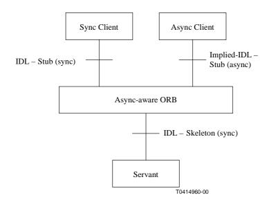
Figure 8/Q.816 – Asynchronous-aware ORB
