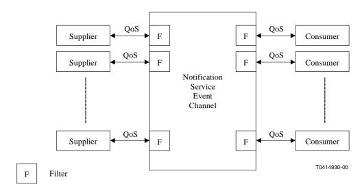
Figure 5/Q.816 – Architecture of the Notification Service
