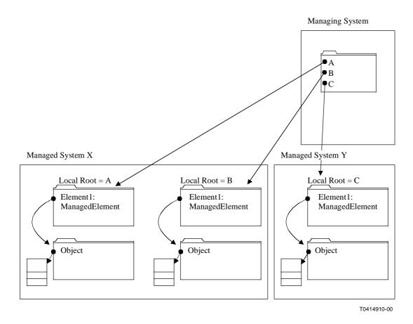
Figure 3/Q.816 – Assigning names to root naming contexts
