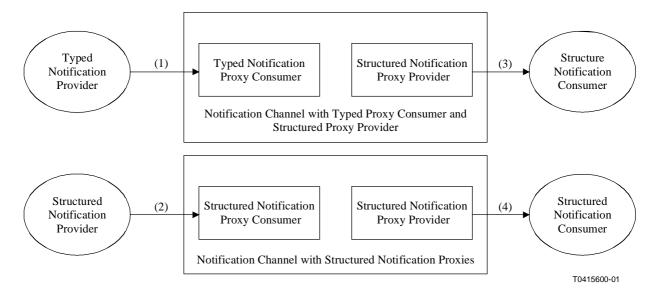
Figure II.1/Q.816 – Example of Typed and Structured Notification Posting, with Structured Delivery
