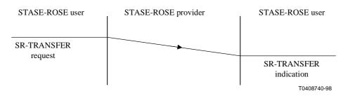
Figure 3/Q.813 – SR-TRANSFER service primitives
