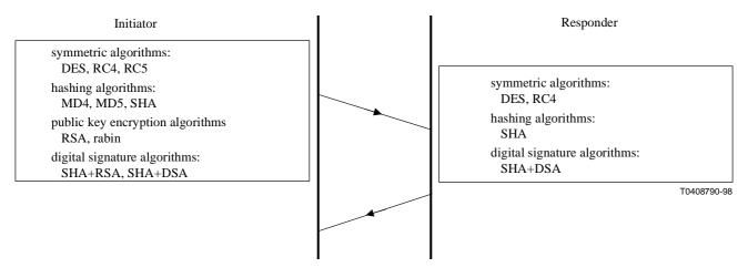
Figure II.1/Q.813 – Negotiation of security algorithms
