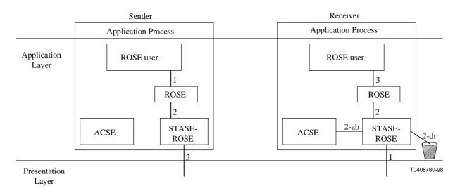
Figure 7/Q.813 – Interaction during data transfer
