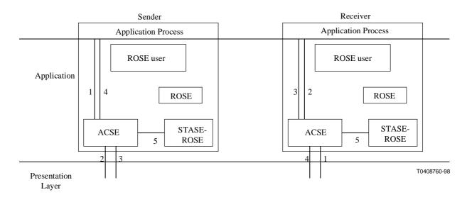
Figure 5/Q.813 – Interaction during association release
