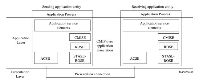
Figure 2/Q.813 – ASEs present when STASE-ROSE is used for securing CMISE
