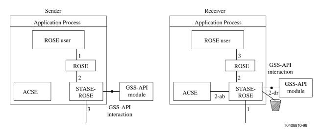
Figure III.2/Q.813 – Use of GSS-API with STASE-ROSE during data transfer
