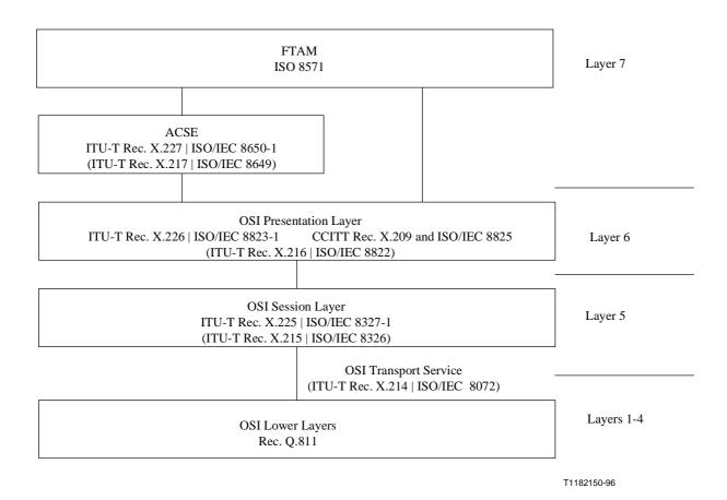
Figure 2/Q.812 – Protocol stack of the upper layer protocol profile for File-oriented Class services
