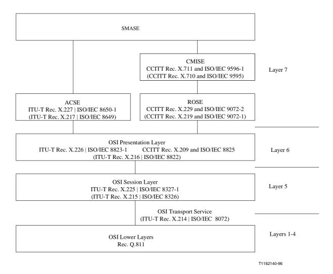
Figure 1/Q.812 – Protocol stack of the upper layer protocol profile for Interactive Class services
