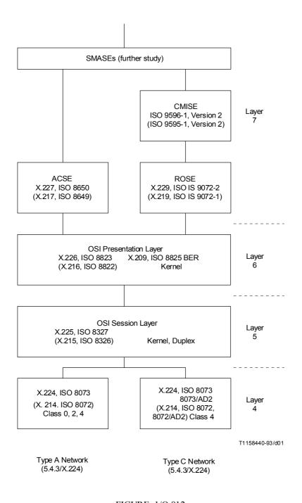
$FIGURE\ 1/Q.812$  Protocol profile for network management which uses transaction function
