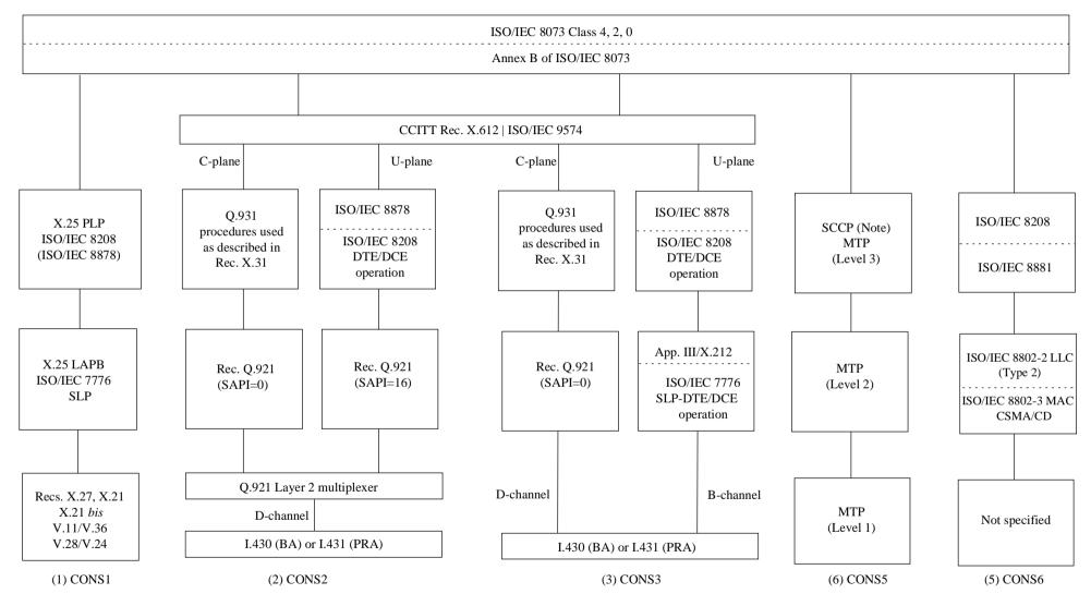
NOTE - Further study is needed for the function of SCCP at the boundary of Network layer and Transport layer.
