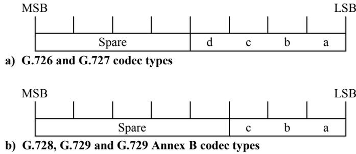
**Figure 16/Q.765.5 – Coding for the 1 octet long configuration field**
