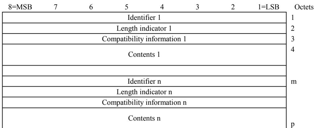
**Figure 7/Q.765.5 – Encapsulated Application Information field**
