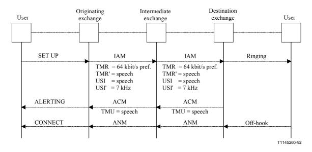
Figure D.4/Q.764 – Fallback when called user is non-ISDN
