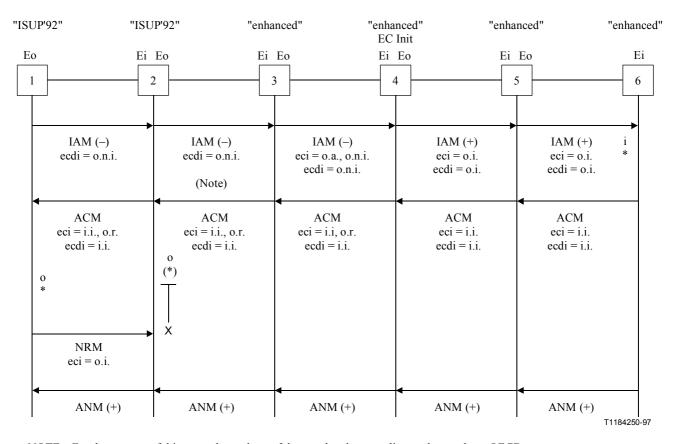
NOTE – For the purpose of this example, exchange 3 knows that the preceding exchanges have OECDs available and consequently passes on the request for that exchange to provide an OECD.
