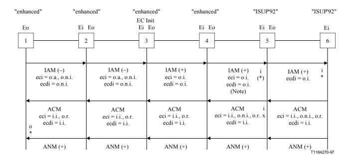
NOTE – The Echo Control Information sent in the IAM from exchange 4 will be an expected parameter at exchange 5. For the purpose of this example, exchange 4 knows that the succeeding exchange has echo cancellers available and does not provide an IECD itself.
