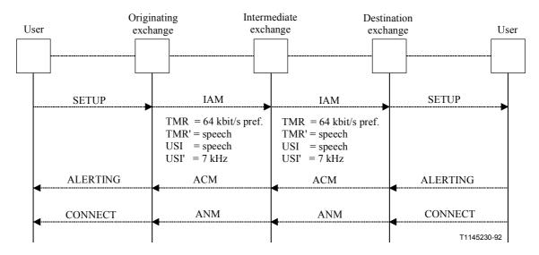
Figure D.1/Q.764 - Fallback does not occur
