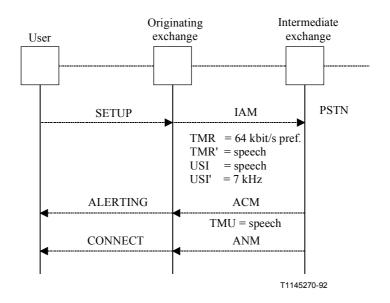
Figure D.5/Q.764 – Fallback when interworking with PSTN
