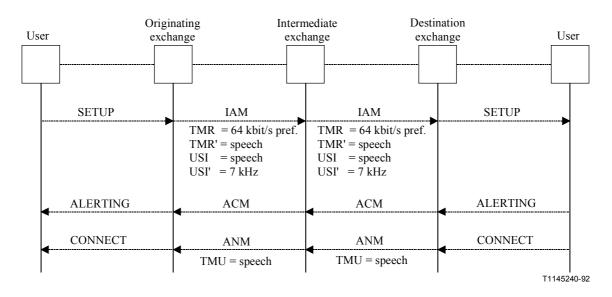
Figure D.2/Q.764 – Fallback occurs to speech at the destination interface – Fallback indicated in connect
